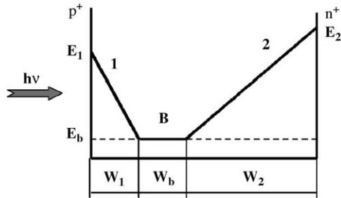
Fig. 4. Electric field distribution in a heavily irradiated Si detector assuming a non-zero electric field in the base region B.
