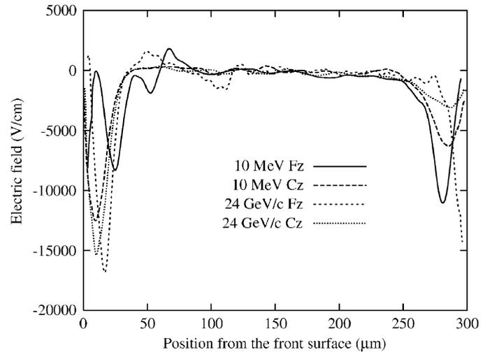
Fig. 7. Electric field distribution in silicon bulk acquired by SEM measurement. The detectors are biased with 40 V. The  $p^+$  contact is on the left and the  $n^+$  contact is on the right.
