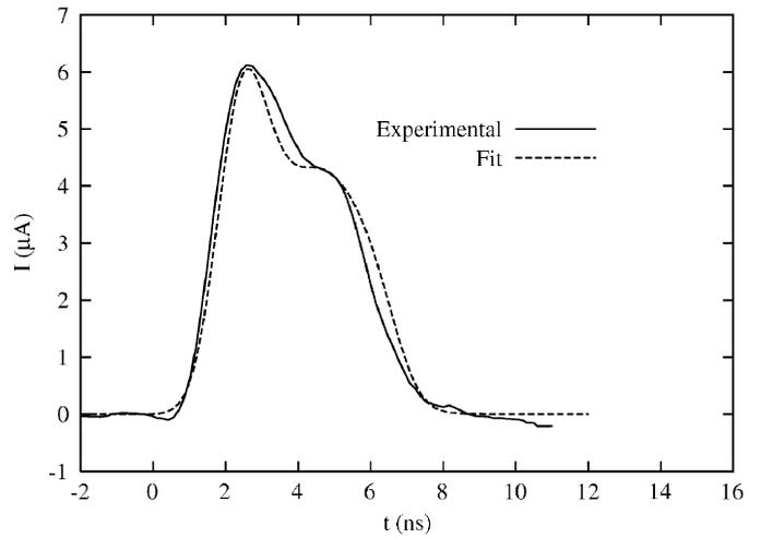
Fig. 5. The experimental pulse response from the  $p^+$  side of the Fz-Si pad detector #56 operated at  $V = 398$  V and the simulated response.
