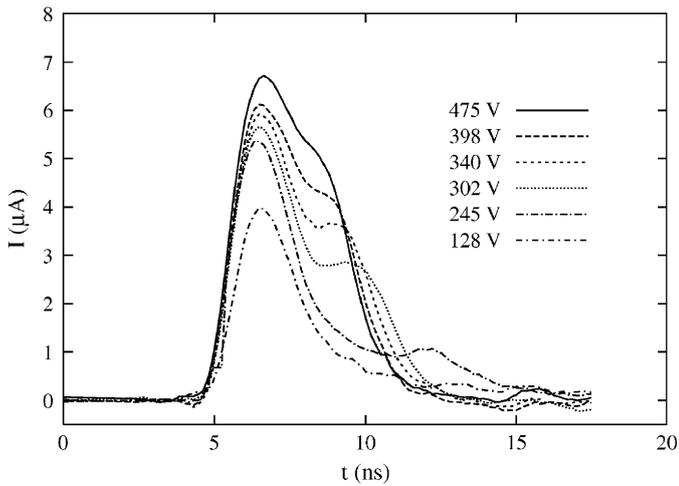
Fig. 3. The TCT curves obtained by illuminating the  $p^+$  contact (front side) of the Fz-Si pad detector #56.
