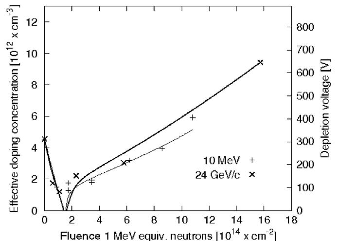
Fig. 1. The evolution of effective doping concentrations ( $N_{\text{eff}}$ ) in Cz-Si pad detectors irradiated with 10 MeV (+) and 24 GeV/c (x) protons.
