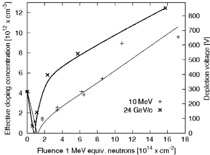
Fig. 2. The evolution of effective doping concentrations ( $N_{\text{eff}}$ ) in Fz-Si pad detectors irradiated with 10 MeV (+) and 24 GeV/c (x) protons.
