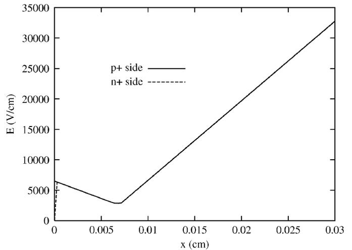
Fig. 6. Electric field distribution reconstructed from the pulse response presented in Fig. 5.
