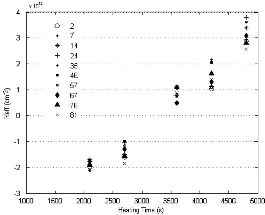
Fig. 2. Effective doping concentration ( $N_{\text{eff}}$ ) with respect to heating time at 430 °C. The individual symbols correspond to the diode numbering presented in Fig. 1.
