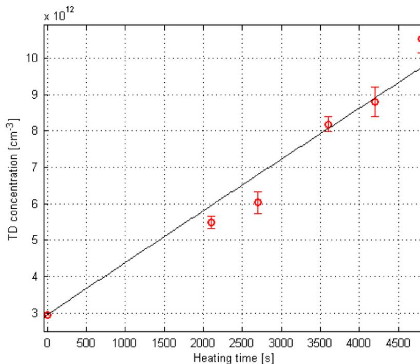
Fig. 3. Exponential fit of the proposed model to the experimental data. The data points correspond to the average of the measurements of  $N_{\text{eff}}$ .
