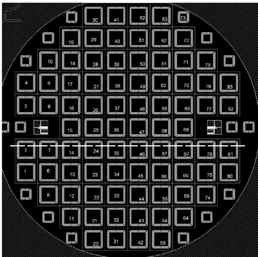
Fig. 1. Position on the wafer of the pad detectors used in this study.
