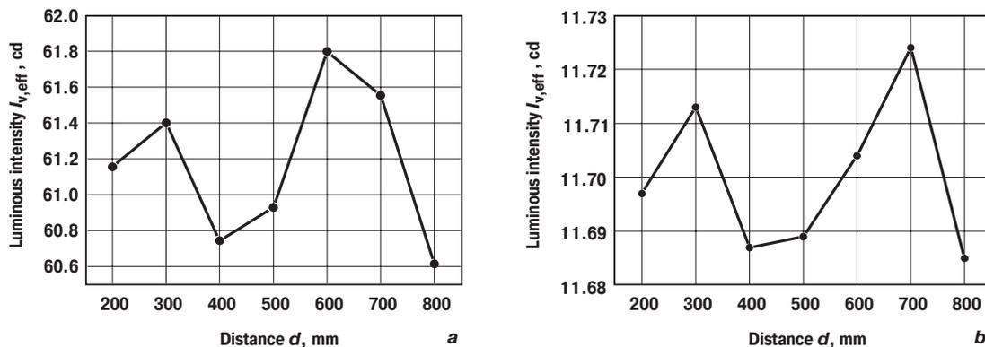
Fig. 3. Luminous intensity  $I_{v,eff}$  as a function of distance for LED #14 (a) and LED #12 (b). The relative peak-to-peak variations of 2 % (a) and 0.3 % (b) are smaller than those in Fig. 1 by a factor of 5 to 20
