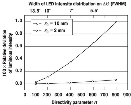
Fig. 4. Relative deviation of the obtained luminous intensity using two different analysis methods. The FWHM width  $\Delta\theta$  of the LED intensity distribution is indicated by the upper scale. The used distance offset was  $\Delta d = 10$  mm
