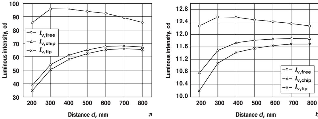
Fig. 1. Luminous intensities  $I_{v,tip}$ ,  $I_{v,chip}$  and  $I_{v,free}$  of LED #14 (a) and LED #12 (b) as a function of distance (see text for details)
