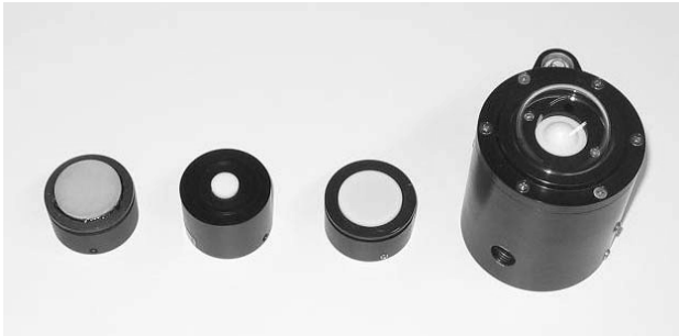
Figure 1. Photograph of the measured spectroradiometer diffusers (from left to right): Bentham D3 (Ø 25 mm), Bentham D7 (Ø 10 mm), Bentham D5 (Ø 23 mm) and Schreder J1002-01 diffuser. (This figure is in colour only in the electronic version)
