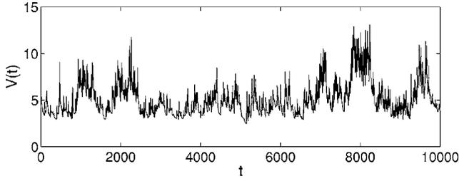
FIG. 1. An example of the time series  $V(t) = \sum_i |v_i|$  from a system of linear size  $L=300b$ ,  $\sigma=0.03$ . Time is reported in units of  $1/(\chi_d Db)$  and  $V$  in units of  $\chi_d Db^2$ . In the steady state, the system contains on the average about 600 dislocations.
