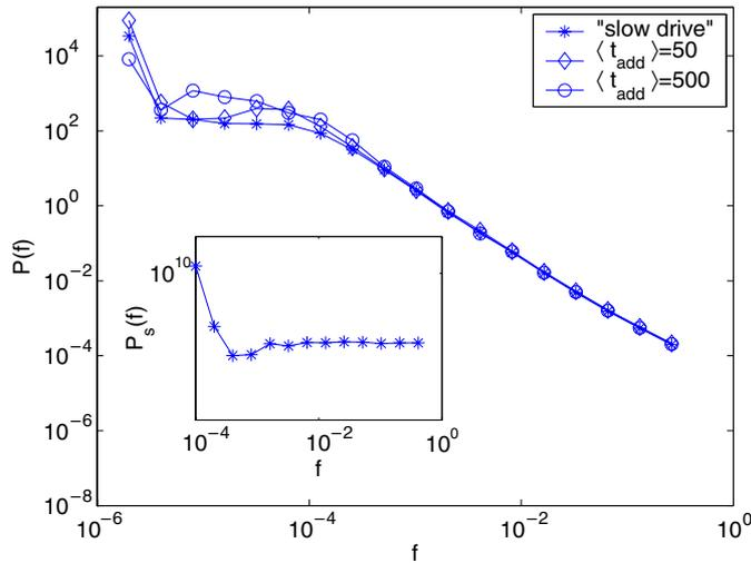
**Figure 1.** Main figure: a comparison of the power spectra of the 2D Manna model,  $L = 256$ , with slow and continuous drives. In the continuous drive case, the time intervals  $t_{\text{add}}$  between successive grain additions are taken from a Poisson distribution with two different averages. Notice how the high frequency part of the PS is independent of the drive. Inset: the power spectrum of the avalanche size time series displaying white noise character.
