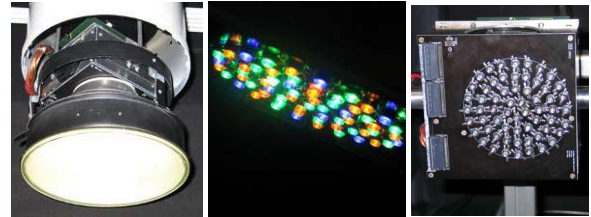
Figure 1. MW-LED fixture with adjustable CCT control
