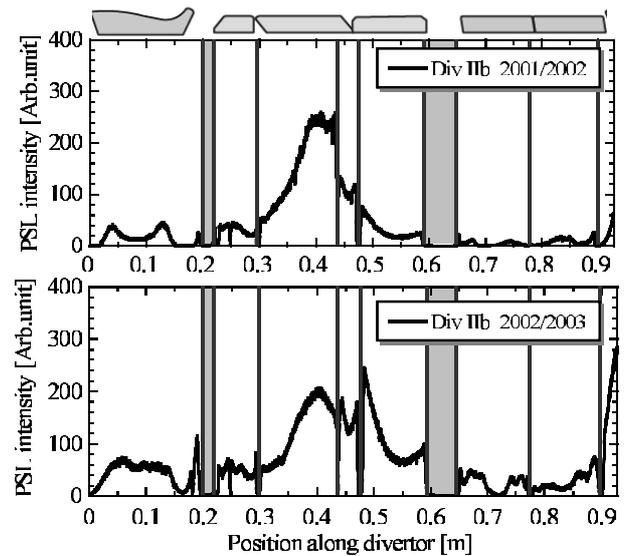
Fig. 2: The measured Photo-Stimulate Luminescence (PSL) intensity on the divertor from ASDEX Upgrade campaigns 2001/2002 and 2002/2003. Reprinted with permission from fig. 24, ref. [12]. © Copyright 2007 by IOP Publishing Limited.
