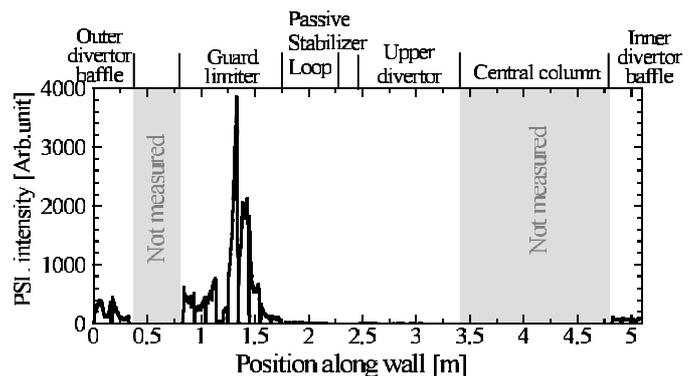
Fig. 3: The measured Photo-Stimulate Luminescence (PSL) intensity on the wall from ASDEX Upgrade campaign 2002/2003. Reprinted with permission from fig. 25, ref. [12]. © Copyright 2007 by IOP Publishing Limited.
