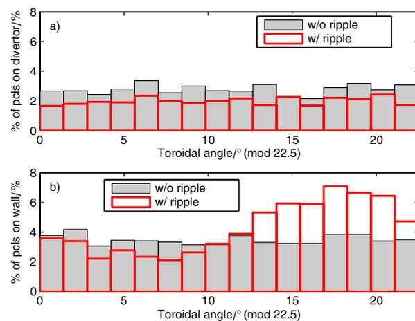
Fig. 5: (Colour on-line) The toroidal distribution of the triton flux a) onto the divertor and b) onto the wall structures in the axisymmetrical case (grey bars) and in the case with finite toroidal ripple (red/grey thick-lined bars). Reprinted with permission from fig. 23, ref. [12]. © Copyright 2007 by IOP Publishing Limited.
