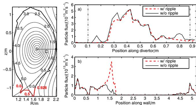
Fig. 4: (Colour on-line) The triton flux a) onto the divertor and b) onto the wall structures in the axisymmetrical case (solid line) and in the case with finite toroidal ripple (red/grey thick dashed line). The strike-points are marked with vertical dash-dotted lines in a), and the coordinates are illustrated on the left. Reprinted with permission from figs. 1 and 22, ref. [12]. © Copyright 2007 by IOP Publishing Limited.
