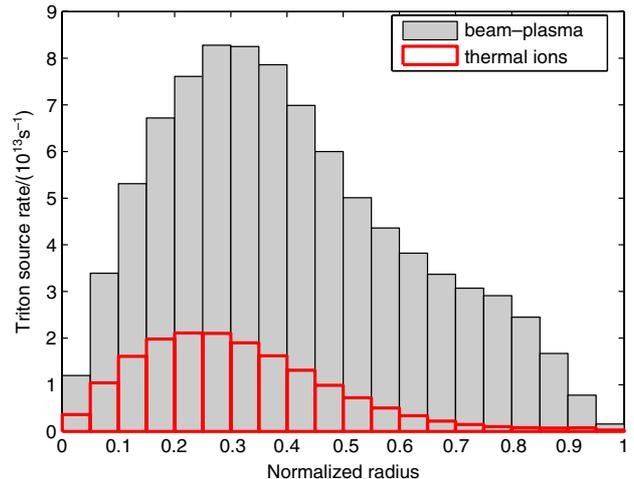
Fig. 1: (Colour on-line) The triton source rate for beam–plasma (grey bars) and thermal (red/grey thick-lined bars) D–D reactions calculated for ASDEX Upgrade shot # 17219. Reprinted with permission from fig. 21, ref. [12]. © Copyright 2007 by IOP Publishing Limited.
