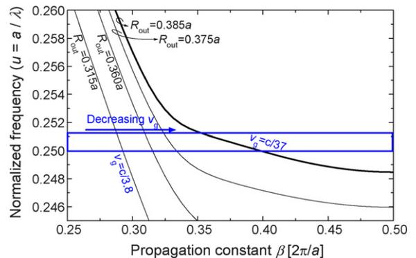
Fig. 2. Dispersion relation of the even mode in RPhCWs with different outer radius  $R_{out}$ . The ring width  $R_{out} - R_{in} = 0.15a$  for all waveguides. In the normalized frequency range within the frame, the average group velocity decreases from  $v_g = c/3.8$  when  $R_{out} = 0.315a$  to  $v_g = c/37$  when  $R_{out} = 0.385a$ .
