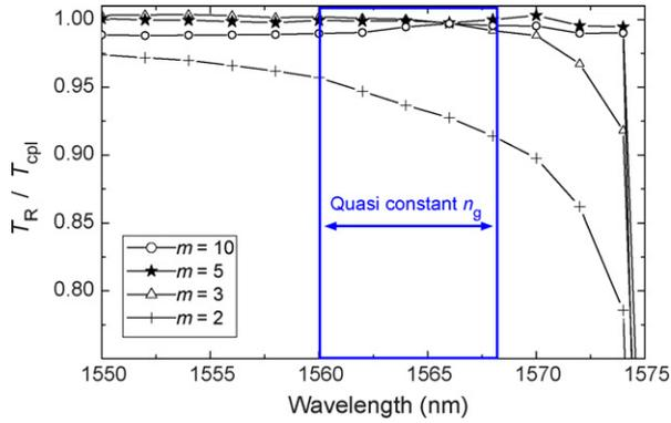
Fig. 7. A measure for mode conversion efficiency,  $T_{\text{opt},R}/T_{\text{cpl}}$ , with different coupler lengths.  $T_{\text{opt},R}$  is the linear interpolation between the points corresponding to F–P resonances in the transmission spectra with a coupler with a length of  $m$  lattice periods, and  $T_{\text{cpl}}$  is the transmission spectra of the coupler sandwiched between strip waveguides.
