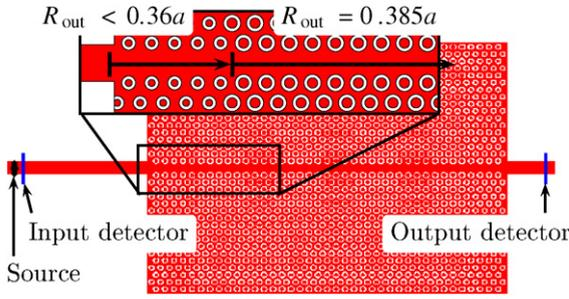
Fig. 3. Schematic image of the coupler design. A slow-light RPhCW is coupled to SWs through RPhCWs with smaller  $R_{\text{out}}$ , i.e., with higher  $v_g$ . The inset shows the beginning of the RPhCW. The source and detector configuration in FDTD simulations is also shown in the schematic.
