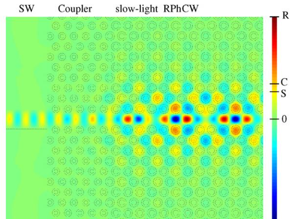
Fig. 5. The  $H_z$  field in the input coupler with a continuous wave source operating at frequency  $u = 0.2506$ . The zero point and maxima of  $H_z$  in the SW (S), coupler (C) and RPhCW (R) are marked onto the colorbar.
