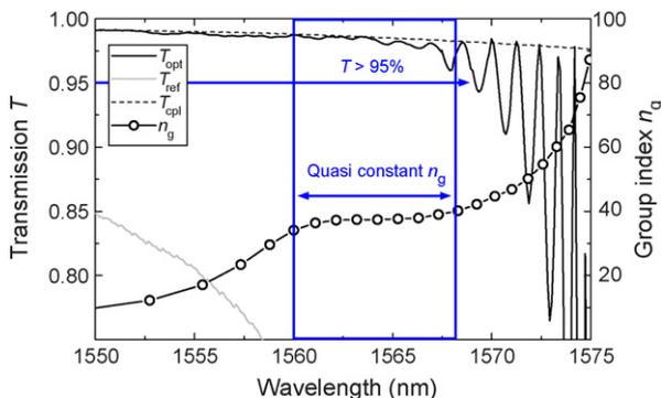
Fig. 6. FDTD simulated transmission spectra through a  $50a$  long RPhC waveguide with  $R_{\text{out}} = 0.385a$  and  $a = 392$  nm, with and without couplers at both ends ( $T_{\text{opt}}$  and  $T_{\text{ref}}$ , respectively).  $T_{\text{cpl}}$  is the transmission spectrum of a  $10a$  long RPhCW with  $R_{\text{out}} = 0.315a$  (i.e., a waveguide similar to the couplers) sandwiched between SWs. Group index  $n_g = c/v_g$  is deduced from the PWE simulations [11].
