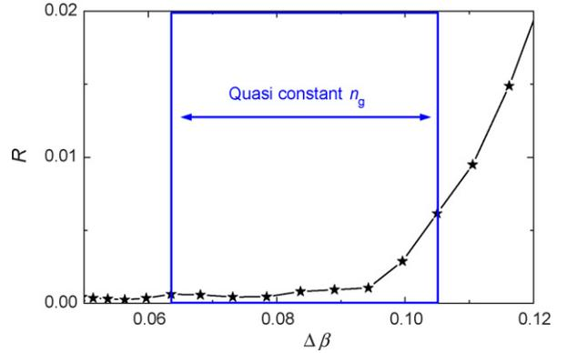
Fig. 8. Parasitic back-reflectance  $R$  as a function of propagation constant mismatch  $\Delta\beta$  with a  $5a$  long coupler. The wavelength range of the figure is from about 1555 to about 1570 nm, the quasi-constant  $n_g$  region is drawn between 1560 and 1568 nm and the scatter symbols have an interval of 1 nm.
