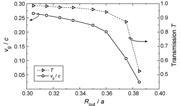
Fig. 4. Group velocity in the RPhCW (solid line) and the transmission of a  $10a$  long RPhCW sandwiched between two strip waveguides (dashed line) as a function of  $R_{\text{out}}$  at the normalized frequency  $u = 0.250$ .
