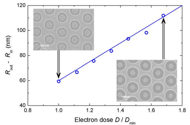
Fig. 8. Measured ring width  $R_{\text{out}} - R_{\text{in}}$  after etching of the RPhC as a function of the electron dose  $D$  applied during electron beam lithography.  $D$  is expressed in Coulombs per unit length in the line exposure mode.  $D_{\text{min}}$  is the smallest dose that yields well-defined rings. The insets are scanning electron micrographs of RPhC patterned with different doses. The period of the RPhC is 440 nm.
