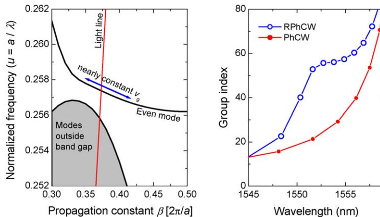
Fig. 5. Dispersion relation and group index in a W1 RPhCW with  $a = 400$  nm,  $R_{\text{out}} = 0.385a$  and  $R_{\text{in}} = 0.235a$ . Group index in a W1 PhCW with  $a = 375$  nm and  $R = 0.305a$  is plotted for reference. For both waveguides,  $f_{\text{air}} \approx 34\%$  and the silicon slab thickness  $h = 1.02a$ .
