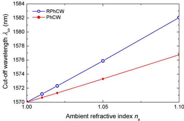
Fig. 6. Calculated cut-off wavelength as a function of the ambient refractive index  $n_a$  for a W1 PhCW and a W1 RPhCW etched in SOI. For the RPhCW:  $a = 405$  nm,  $R_{\text{out}} = 0.385a$  and  $R_{\text{in}} = 0.235a$ . For the PhCW:  $a = 380$  nm and  $R = 0.305a$ . For both waveguides  $f_{\text{air}} \approx 34\%$  and  $h = a$ .
