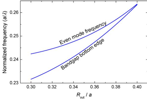
Fig. 4. Frequencies of the bandgap bottom edge and the even guided mode at  $\beta = 0.35(2\pi/a)$  as a function of ring outer radius  $R_{\text{out}}$  in a W1 RPhCW with a ring width  $R_{\text{out}} - R_{\text{in}} = 0.15a$ , in a silicon slab with a thickness  $h = 1.02a$ .
