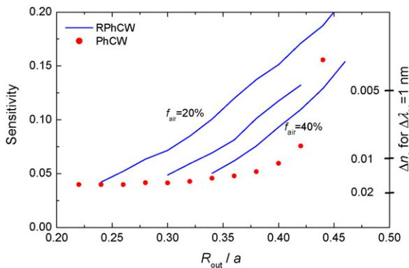
Fig. 7. Calculated sensitivity in RPhCW with  $f_{\text{air}} = 20\%$ , 30% and 40%. The dots correspond to a conventional PhCW with hole radius  $R_{\text{out}}$ . The sensitivity is defined as the relative cut-off shift  $\Delta\lambda_{\text{co}}/\lambda_{\text{co}}$  in % induced by an ambient refractive index change  $\Delta n_a$  equal to 0.01. The ticks on the y axis on the right show  $\Delta n_a$  that induces  $\Delta\lambda_{\text{co}} = 1$  nm when  $\lambda_{\text{co}} = 1570$  nm.
