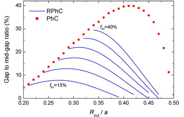
Fig. 3. Gap to mid-gap ratio for the TE polarization in an RPhC as a function of ring outer radius  $R_{\text{out}}$ . The solid lines correspond to air-fill factors from 15% to 40% with a step of 5% units. The dots correspond to a conventional PhC.
