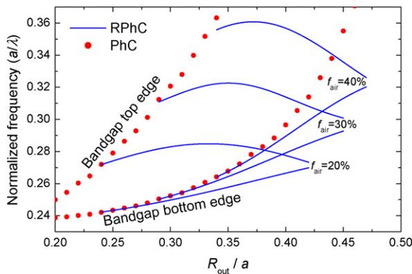
Fig. 2. Bandgap top and bottom edge frequencies for the TE polarization in an RPhC as a function of ring outer radius  $R_{\text{out}}$  at different air-fill factors. The dots correspond to a conventional PhC with radius  $R_{\text{out}}$  ( $R_{\text{in}} = 0$ ).
