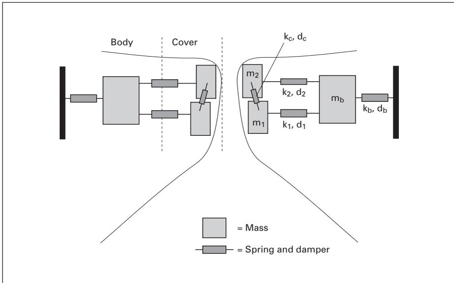
**Fig. 2.** Diagram of the three-mass model of the vocal fold cover-body structure. The cover is represented by the masses  $m_1$  and  $m_2$ , and the body by  $m_b$ . The masses are coupled by stiffness and damping elements.
