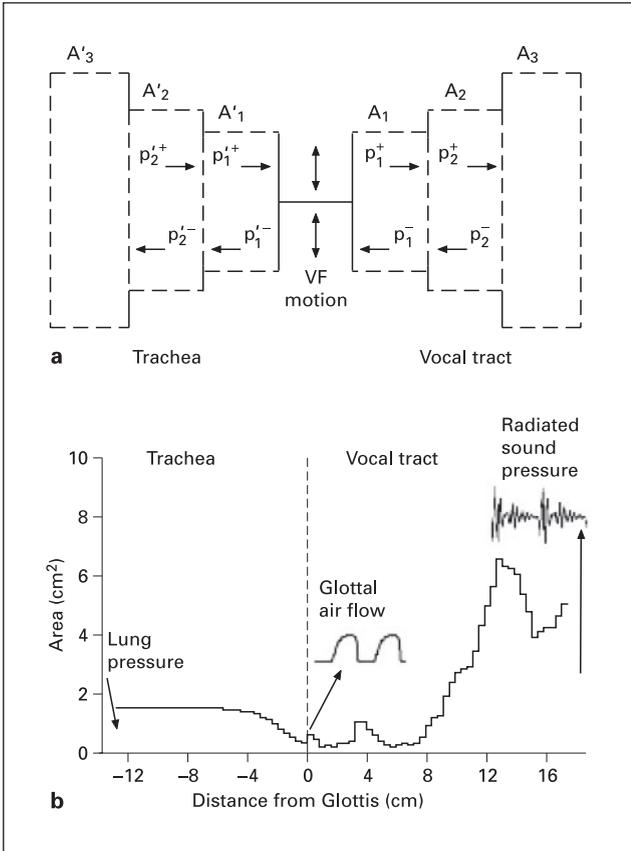
**Fig. 3.** Example of propagating acoustic pressures with a wave reflection model. **a** Tubular idealization of the upper portion of the trachea and lower portion of the vocal tract with forward ( $p^+$ ) and backward ( $p^-$ ) travelling partial pressures. Note that the vocal fold model is assumed to be operating at the point labelled ‘VF motion’. **b** Sample area function of the tracheal/vocal tract system. Glottal air flow and radiated sound pressure signals are also shown.
