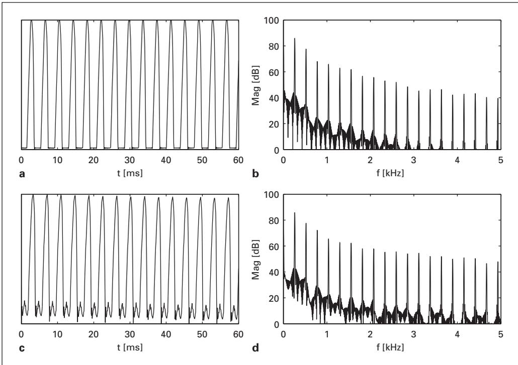
**Fig. 5.** Examples of flow waveforms and their power spectra ( $F_0 = 260$  Hz). Upper graphs: the original glottal flow computed by physical modelling (a) and its power spectrum (b). Lower graphs: the flow waveform (c) and its power spectrum (d) estimated from the speech pressure waveform (vowel /ae/) with inverse filtering.
