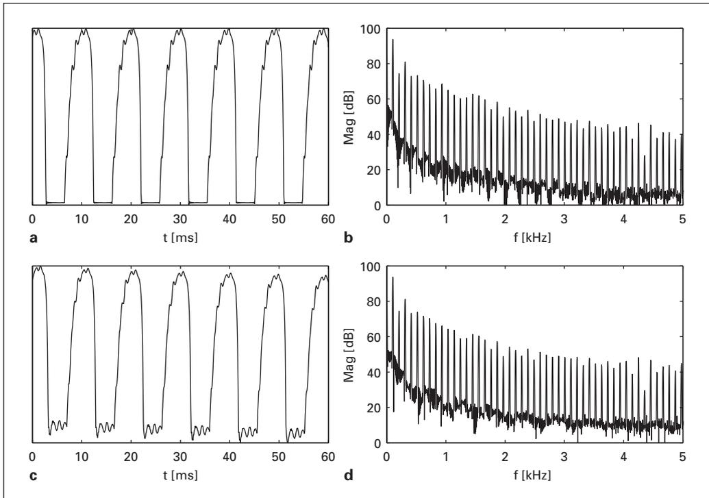
**Fig. 4.** Examples of flow waveforms and their power spectra ( $F_0 = 100$  Hz). Upper graphs: the original glottal flow computed by physical modelling (a) and its power spectrum (b). Lower graphs: the flow waveform (c) and its power spectrum (d) estimated from the speech pressure waveform (vowel /a/) with inverse filtering.
