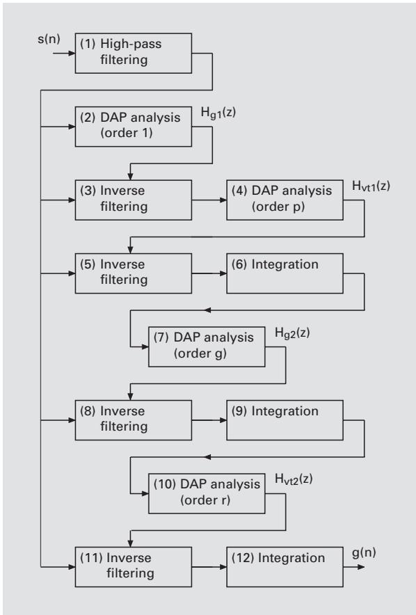
**Fig. 1.** Block diagram of the IAIF method. The input of the method is the speech pressure signal, denoted by  $s(n)$ , from which the inverse filtering algorithm estimates the glottal volume velocity waveform, denoted by  $g(n)$ .
