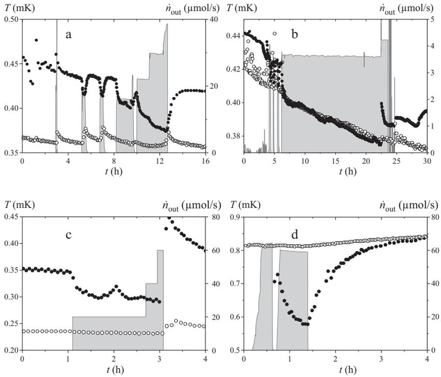
**Fig. 2.3** Four examples of the adiabatic melting cooling, see text for details. The temperature scale is shown on the left. The sample temperature, measured by a vibrating wire in pure  $^3\text{He}$  phase is shown by the filled symbols and the temperature of the cell wall by the open ones. The filled gray area shows the flow through the superleak, the scale being given on the right. The time axis shows the time in hours from an arbitrary point close to the start of melting attempt.
