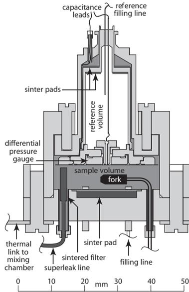
**Fig. 3.1** Cross section of the detached pressure gauge used as experimental cell in osmotic pressure and solubility measurements. The capacity of the sample volume was  $8.3 \pm 0.2 \text{ cm}^3$  and that of the reference volume  $18 \text{ cm}^3$ .
