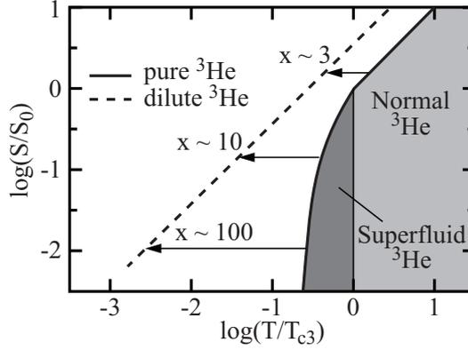
**Fig. 2.1** Molar entropy of  $^3\text{He}$  in pure and dilute phases. The arrows indicate perfectly adiabatic transitions from different starting temperatures, resulting in cooling factors  $x = T_{\text{initial}}/T_{\text{final}}$ .
