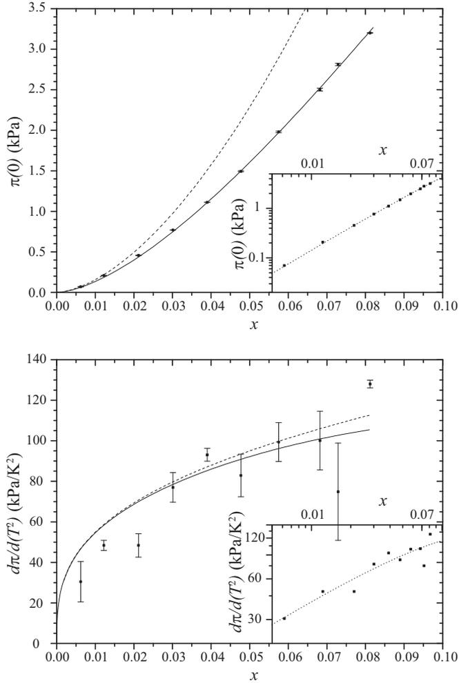
**Fig. 3.3** Osmotic pressure at zero temperature (top) and coefficient of quadratic temperature dependence (bottom) as a function of concentration. The symbols with error bars are the measured values, the solid lines are results of a theoretical calculation using a fitted interaction potential for the quasiparticles, and the dashed lines are results when the interactions are omitted. The insets show the same data on logarithmic scales along with semiempirical fits.
