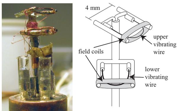
**Fig. 2.5** A photograph and a schematic drawing of the vibrating wire resonator insert used in the adiabatic melting experiment. The upper wire is made of 50  $\mu\text{m}$  diameter NbTi and the lower of 125  $\mu\text{m}$  Ta filament.
