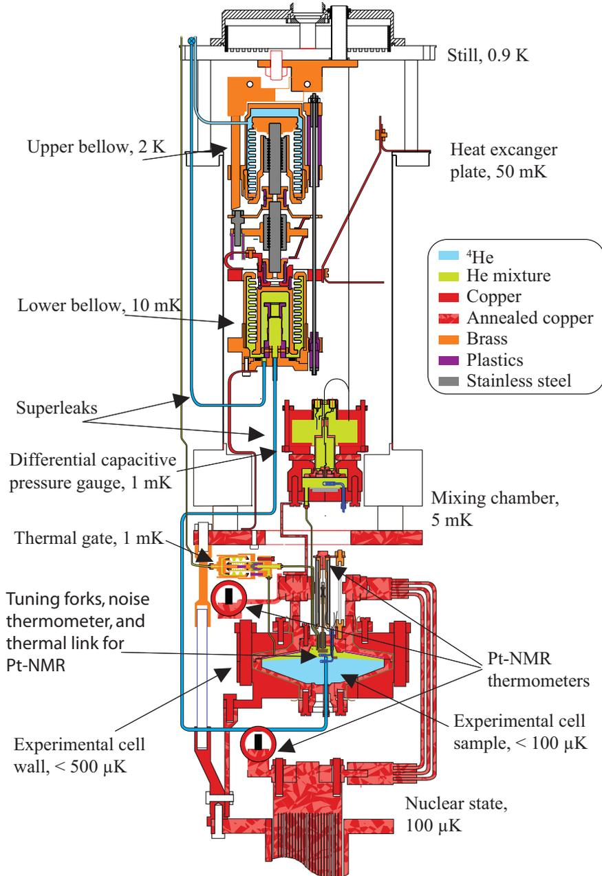
**Fig. 2.4** Experimental setup for the adiabatic melting experiment.
