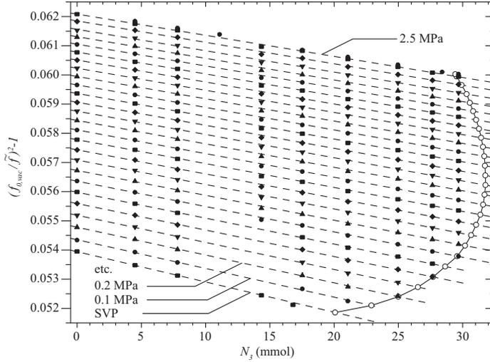
**Fig. 3.2** The density of the  $^3\text{He}/^4\text{He}$  mixture indicated as a change in the idealized resonance frequency  $\tilde{f}$  of the tuning fork as a function of the added  $^3\text{He}$  for selected pressures. The open symbols show the response in saturated mixture, the closed symbols for homogenous mixtures, and the dashed lines are fits to each pressure.
