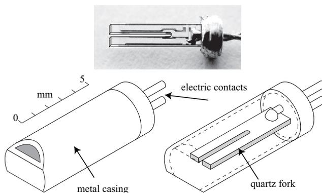
**Fig. 2.6** A photograph and schematic drawing of a quartz tuning fork (Fox Electronics NC38). The outline of the fork in the photograph has been enhanced by drawn lines. The basic geometry is similar also for the smaller fork models used.
