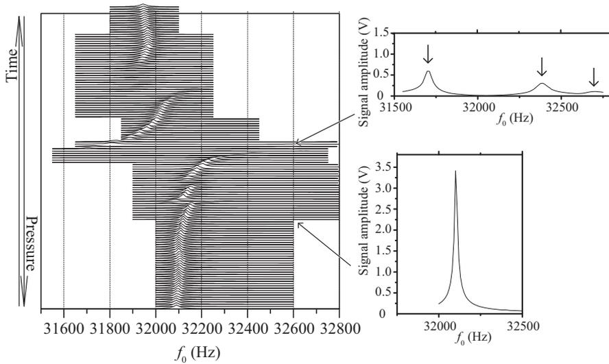
**Fig. 2.7** Acoustic resonances in supercritical  $^4\text{He}$ . The spectra were recorded at the constant temperature of 4.6 K while the pressure decreased from 0.26 to 0.21 MPa in 8 hours. The two inserts show example spectra in situations where no acoustic modes are present (lower frame) and where two acoustic modes are coupled to the mechanical oscillator (upper frame).
