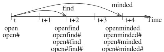
Figure 1: Local acoustic search, stacks, and hypotheses. The two acoustically most probable fragments find and minded are used to expand the two hypotheses at frame  $t$ . The resulting hypotheses are placed in stacks according to the best ending times. The hypotheses comprise all combinations including and excluding word breaks (#).
