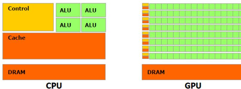
Figure 1: Comparison of CPU and GPU architectures [3].
