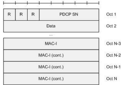
Figure 4: PDCP Data PDU format for SRBs [7].
