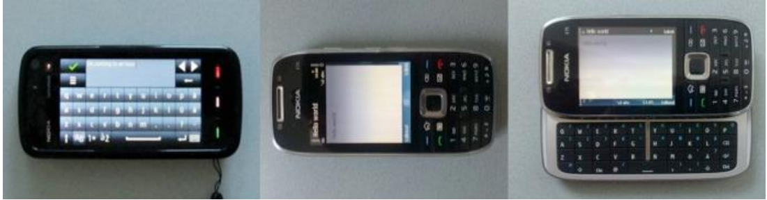
Figure 3. Text input interfaces compared in the study. From left: Touch-Qwerty keyboard, ITU-12 keypad and Physical-Qwerty keyboard.
