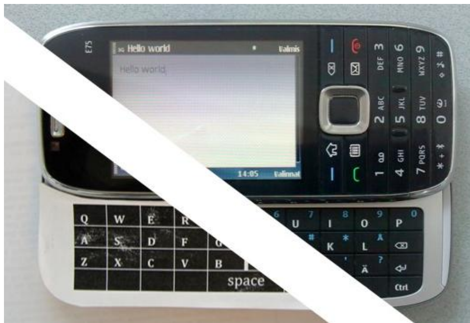
Figure 5. A thin layer of plastic with printed key layouts on the keyboard (left) was used to block feedback from the button edges and key releases of the original keyboard (right).
