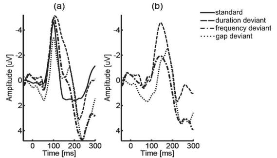
FIG. 6. An example of the responses recorded (test subject 2). (a) Average responses to the standard sound and the deviant sounds (duration, frequency, and gap). (b) Difference of the average response to the standard sound and the average response to each of the deviant sounds. The mismatch negativity appears as a peak in the difference curves at the latency of 140 to 175 ms, depending on the type of the deviant sound.
