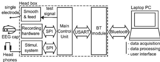
FIG. 1. The block diagram of the prototype system. The audio stimulation system, EEG recording hardware, and the contact tester are integrated into the head box. The user interface and the data processing system are in the PC interface. Communication between the devices takes place via bluetooth (BT).
