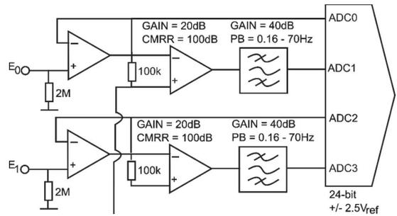
FIG. 3. Two channels of the eight-channel EEG amplifier. The nominal gain in the EEG channels (ADC1, ADC3, etc.) is 60 dB and the passband (PB) is 0.16 to 70 Hz. The input impedance is 2 MΩ. The unamplified channels (ADC0, ADC2, etc.) are used in the contact impedance measurement.
