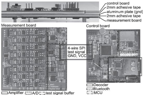
FIG. 5. Packing and layout of the electronics in the head box. The design is divided into two modules: a measurement board and a control board. These are stacked and a metal plate is placed in between them to prevent digital cross talk.
