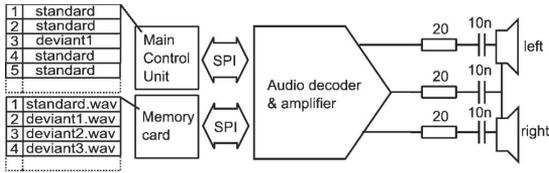
FIG. 4. Audio stimulation system. The order of the stimuli is stored in the memory of the main control unit, which controls the audio decoder that generates the audio signal. Audio files are saved on a memory card.
