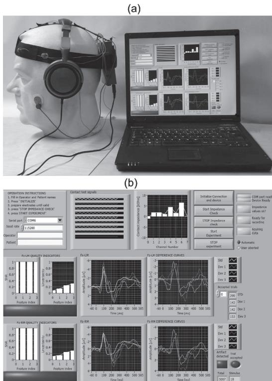
FIG. 2. The prototype implemented and the user interface. (a) The head box is battery powered and wireless and it can be attached to the electrode cap during the experiment. The dimensions are small (96 × 128 × 32 mm<sup>3</sup>; weight: 374 g). (b) The PC interface provides basic operator functions and allows the average waveforms to be processed and monitored online.
