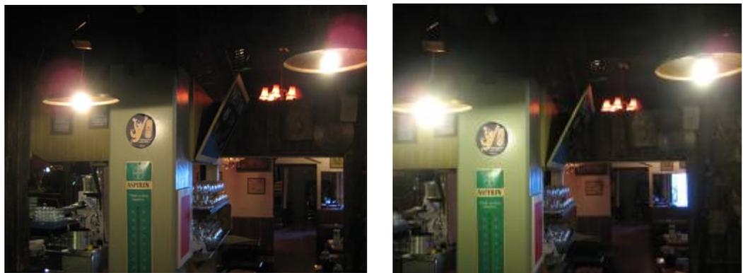
**Figure 4-16.** Effect of lighting with two 40 W incandescent lamps and two 8 W CFLs at the entrance of the room.
