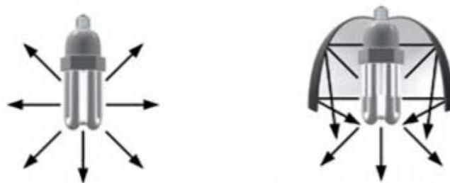
**Figure 3-2.** *Omni-directional light and 0.58 UF of CFL for downward task lighting (Mondoarc 2008).*
