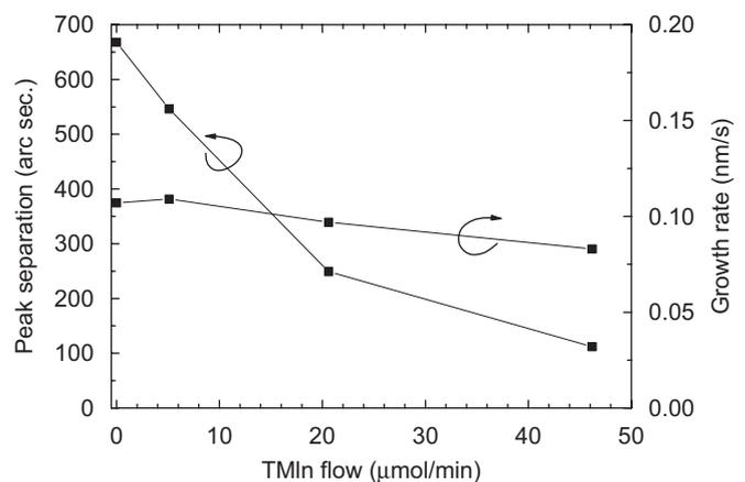
Fig. 2. The InAlGaN and GaN XRD peak separation and growth rate of the InAlGaN films as a function of TMIIn molar flow.
