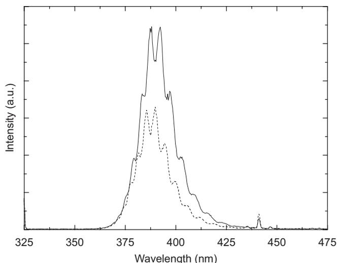
Fig. 5. Room temperature PL spectra of InGaN/InAlGaN MQW samples. Sample A is marked with solid line and sample B with dashed line.
