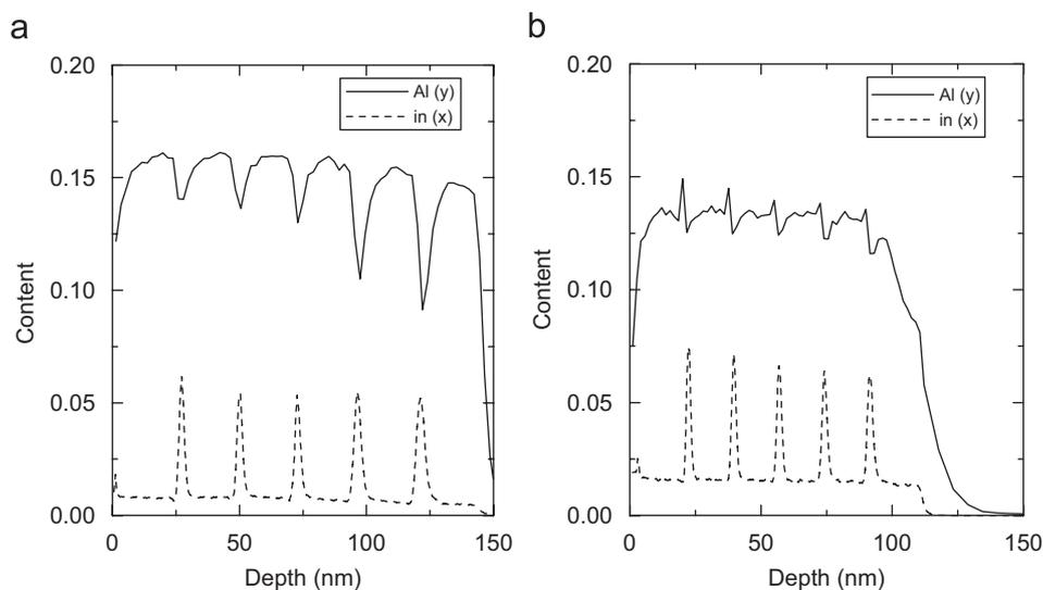
Fig. 4. The In and Al composition depth profiles measured by SIMS of InGaIn/In<sub>x</sub>Al<sub>y</sub>Ga<sub>1-x-y</sub>N MQW samples. TMIn flow of (a) 5  $\mu\text{mol}/\text{min}$  (sample A) and (b) 46  $\mu\text{mol}/\text{min}$  (sample B) were used during the growth of the InAlGaIn barriers.
