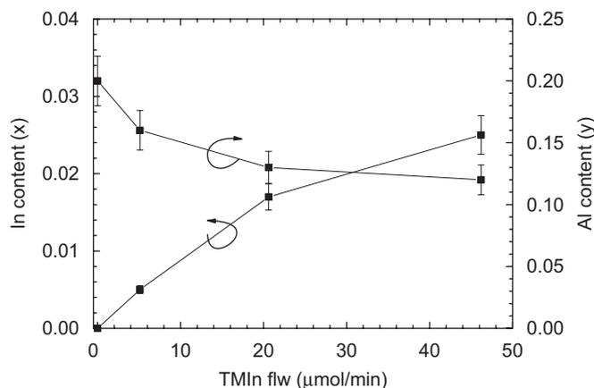
Fig. 3. The In and Al contents of  $\text{In}_x\text{Al}_y\text{Ga}_{1-x-y}\text{N}$  films as a function of TMIn flow.
