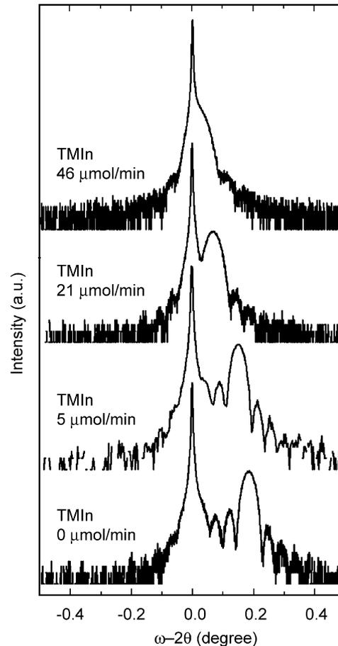
Fig. 1. HRXRD ( $\omega - 2\theta$ ) curves of the (0002) reflections from InAlGaN films grown with various TMIIn flows.
