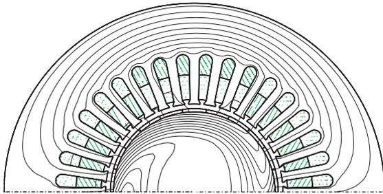
Fig. 1. Flux distribution in the computed geometry of Motor I.
