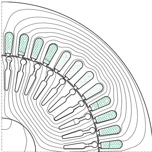
Fig. 2. Flux distribution in the computed geometry of Motor II.
