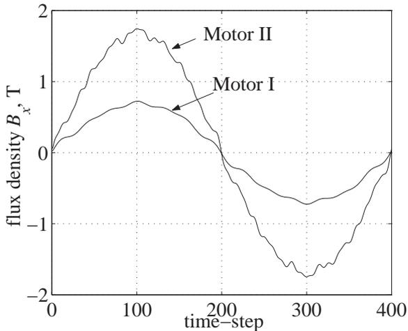
Fig. 3. The flux density waveforms in the teeth of the stator core.
