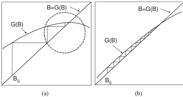
Fig. 1. A comparison of the speed of the fixed-point iteration between the two methods. (a) The local-coefficient method (LCM). (b) The global-coefficient method (GCM).
