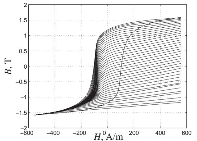
Fig. 2. First-order reversal curves  $H = F(B)$  extrapolated to ensure continuity at the reversal points.
