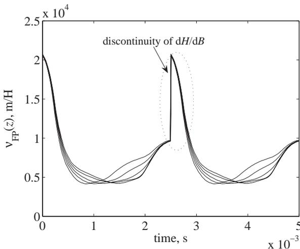
Fig. 4. The variation of the local-coefficient  $\nu_{FP}(z)$  in certain points of the lamination at 200 Hz.
