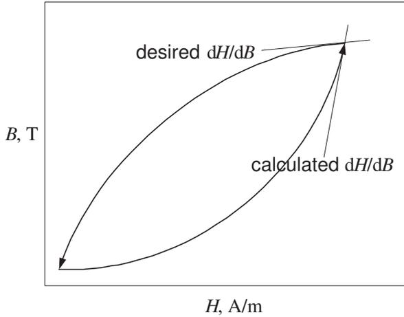
Fig. 3. The difference between the calculated slope and the desired one at a reversal point.
