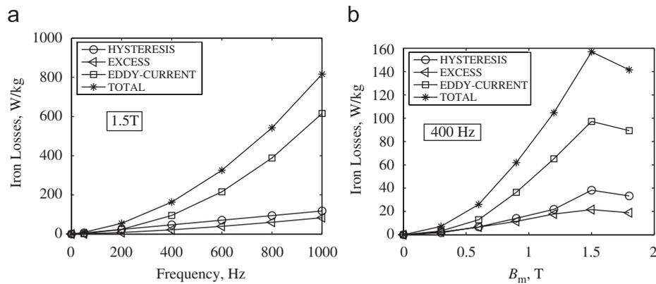
Fig. 5. Separation of the calculated iron losses under circular flux excitation.
