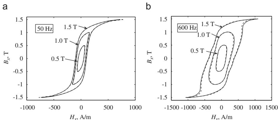
Fig. 1. Measured (solid) and calculated (dashed) unidirectional dynamic loops.
