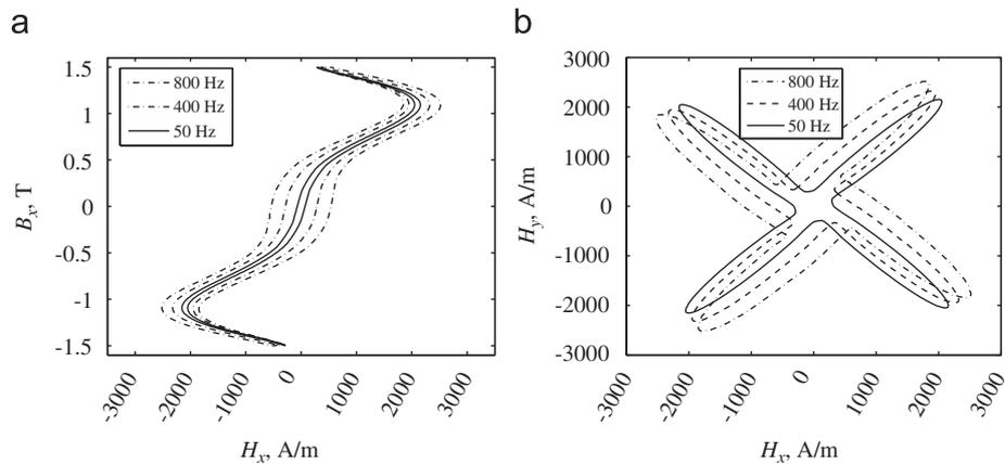
Fig. 4. Dynamic loops calculated under circular flux excitation.
