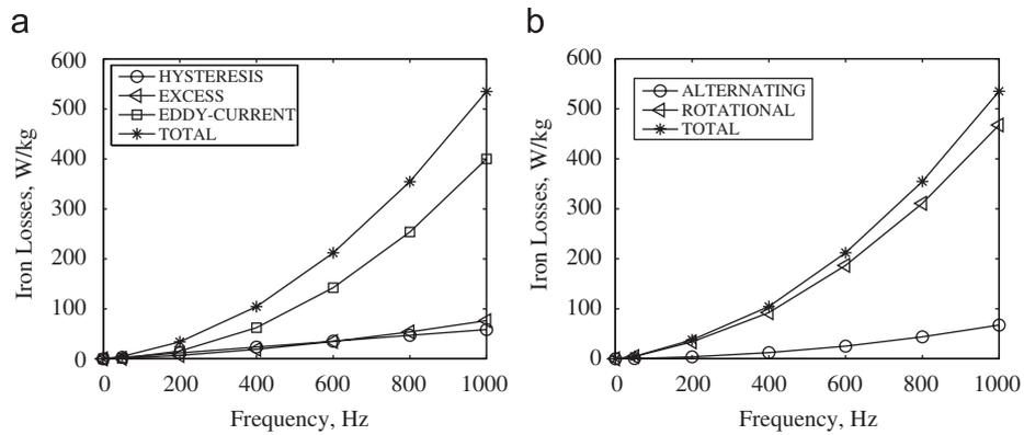
Fig. 3. Separation of the calculated iron losses under elliptic flux excitation shown in Fig. 2a.
