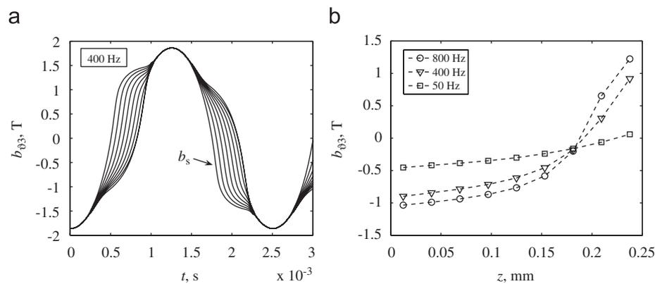
Fig. 6. Flux distribution inside the lamination for  $\theta_3$ .
