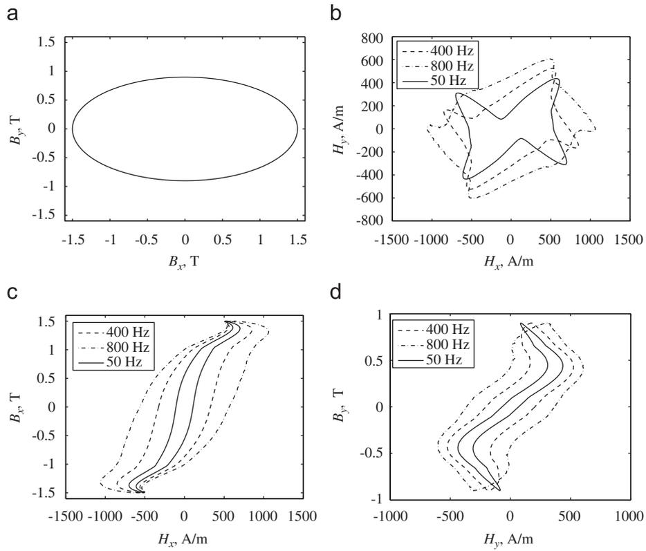
Fig. 2. Dynamic loops calculated under elliptic flux excitation.
