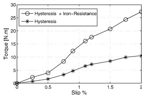
**Fig. 8** Simulations of the iron-resistance torque and the hysteresis torque at varied slips
