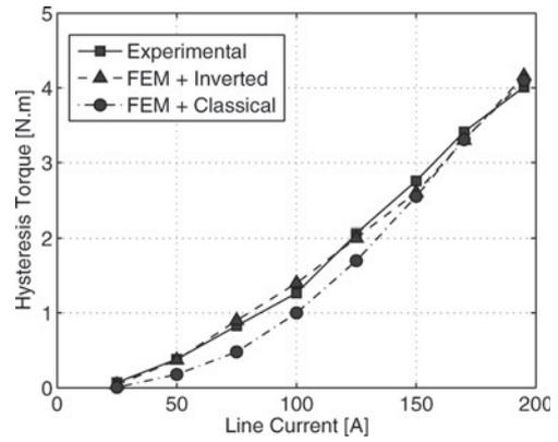
**Fig. 5** Experimental hysteresis torque values compared with the computed ones by the FEM analysis integrated with the inverted Preisach model and the classical Preisach model
