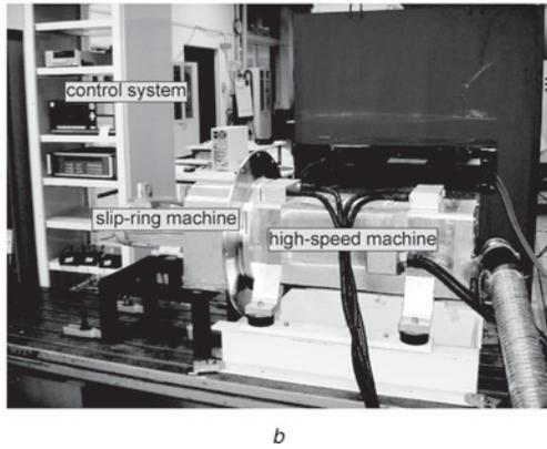
**Fig. 3** Experimental setup for measuring hysteresis torque in the high-speed induction machine
