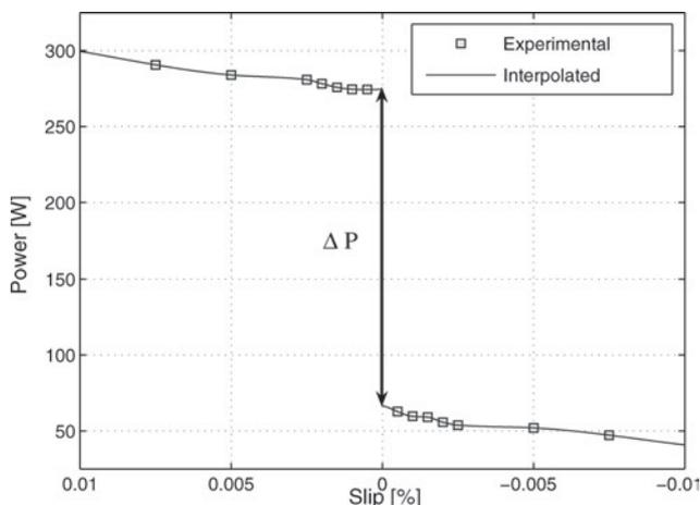
**Fig. 4** Average powers measured as a function of the slip
