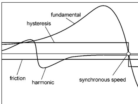
**Fig. 2** Representation of the torque components (fundamental, harmonic, friction, and hysteresis) produced by an induction machine
