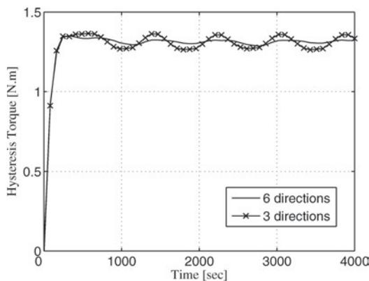
**Fig. 6** Instantaneous hysteresis torque computed by the inverted Preisach vector model incorporated into FEM model at slip 0.001%
