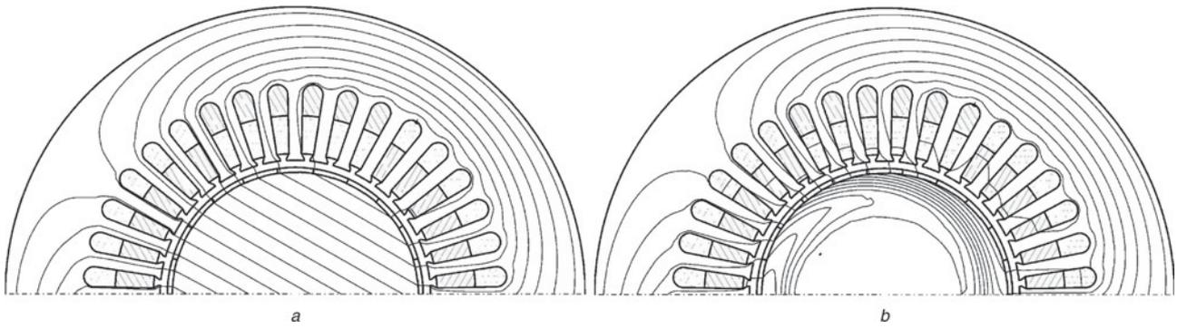
**Fig. 1** Flux distribution in the high-speed induction machine
