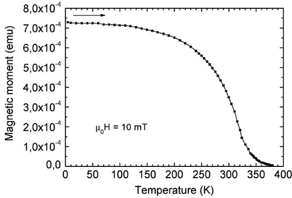
Fig. 6. Magnetization as a function of temperature in (Ga, Mn)N.
