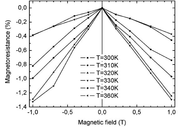
Fig. 3. Magnetoresistance versus magnetic field at various temperatures in (Ga, Mn)N.
