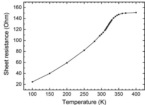
Fig. 5. Sheet resistance as a function of temperature in (Ga, Mn)N.
