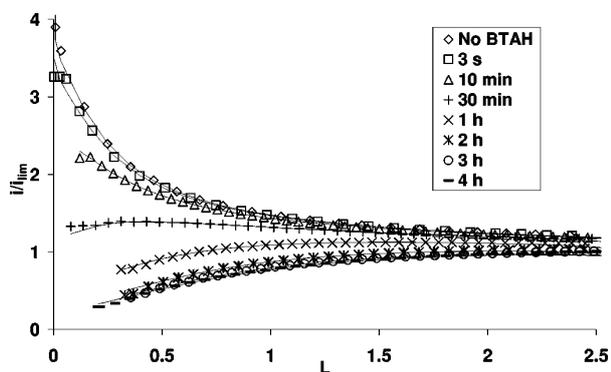
**Figure 1.** The approach curves measured at the substrate potential of  $-0.05$  V vs. SCE.  $i/i_{\text{lim}}$  is the dimensionless tip current, and  $L = d/a$  is the dimensionless distance between the sample and the tip.
