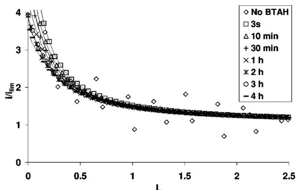
**Figure 5.** The approach curves measured at the substrate potential of  $-0.3$  V vs. SCE.  $i/i_{\text{lim}}$  is the dimensionless tip current, and  $L = d/a$  is the dimensionless distance between the sample and the tip.
