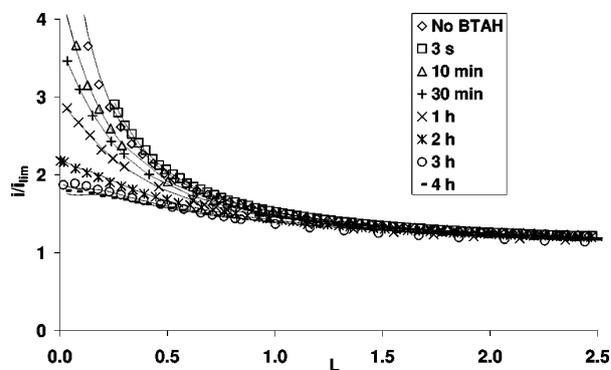
**Figure 2.** Approach curves measured at the substrate potential of  $-0.10$  V vs. SCE.  $i/i_{\text{lim}}$  is the dimensionless tip current, and  $L = d/a$  is the dimensionless distance between the sample and the tip.
