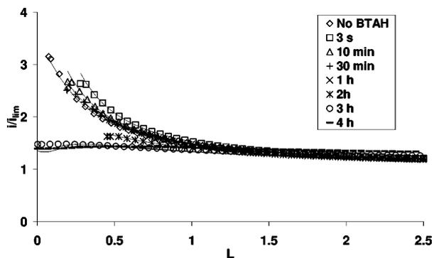
**Figure 3.** The approach curves measured at the substrate potential of  $-0.15$  V vs. SCE.  $i/i_{\text{lim}}$  is the dimensionless tip current, and  $L = d/a$  is the dimensionless distance between the sample and the tip.
