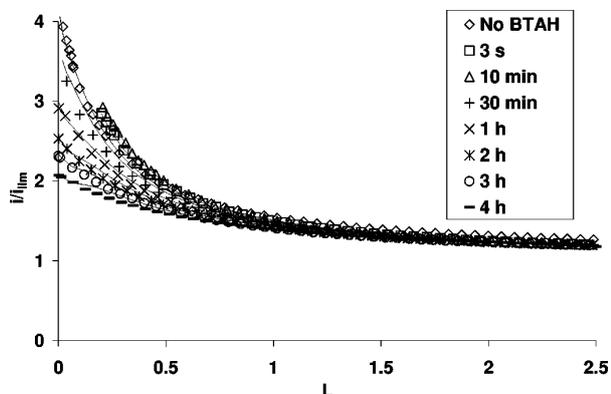
**Figure 4.** The approach curves measured at the substrate potential of  $-0.20$  V vs. SCE.  $i/i_{\text{lim}}$  is the dimensionless tip current, and  $L = d/a$  is the dimensionless distance between the sample and the tip.
