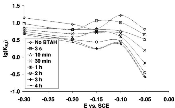
**Figure 8.** Logarithm of the dimensionless rate constant of the mediator at the substrate surface  $K_{S,f}$ , as a function of the substrate potential.  $K_{S,f}$  can be calculated from the modeling result of the approach curves that are measured both as a function of exposure time to BTAH as well as a function of potential of the substrate.
