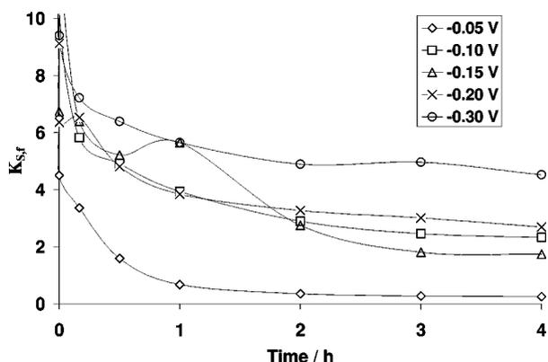
**Figure 7.** Dimensionless rate constant of the mediator at the substrate surface,  $K_{S,f}$ , as a function of the exposure time.
