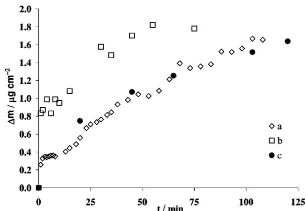
**Figure 9.** Mass increase due to BTAAH adsorption on the copper surface: (a and c) copper is deposited from the solution on the initially unpolished Au crystal, (b) copper is deposited from the solution on the initially polished Au crystal.
