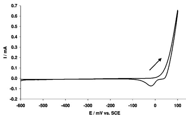
**Figure 6.** The CV of DHP copper measured in 1 mM FcMeOH + 0.1 M  $\text{Na}_2\text{SO}_4$  solution. The sweep rate is 1 mV/s.
