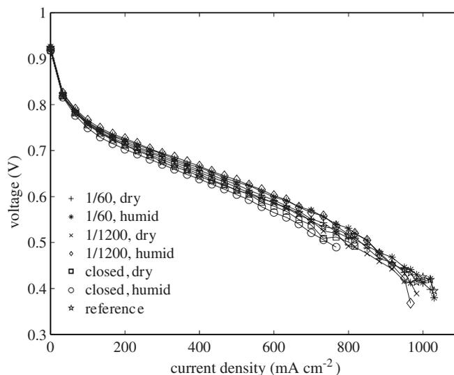
Fig. 2. Polarization curves measured with 0.1 barg hydrogen pressure.
