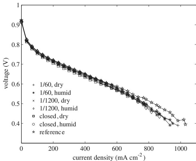
Fig. 3. Polarization curves measured with 0.25 barg hydrogen pressure.
