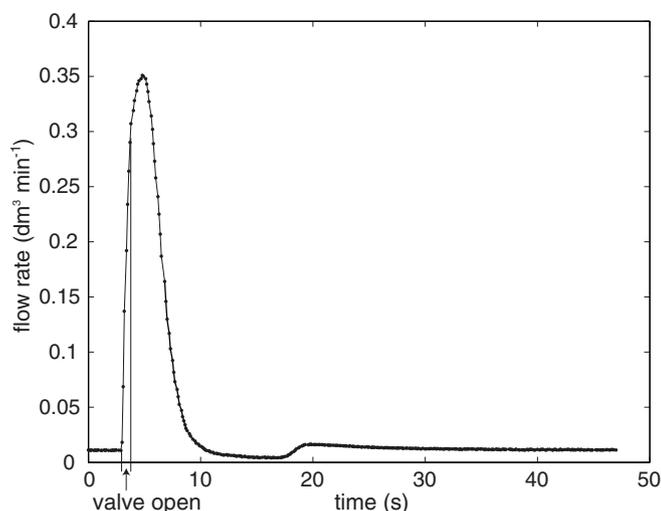
Fig. 6. Hydrogen flow rate during purge.
