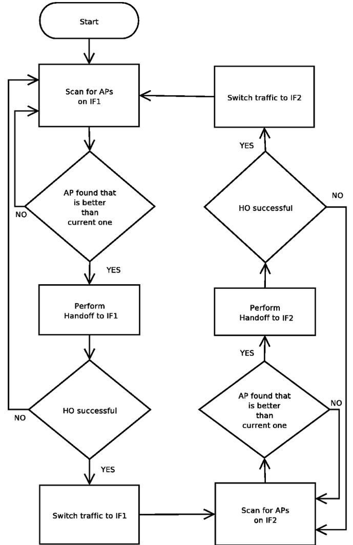
Fig. 2. MBB handoff algorithm with two interfaces.
