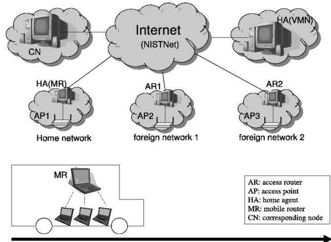
Fig. 1. Logical network topology of the testbed.
