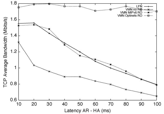
Fig. 7. TCP performance comparison in static case.
