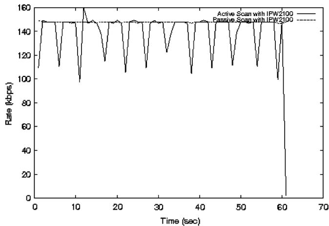
Fig. 3. Effects of active scanning on UDP downstream traffic.
