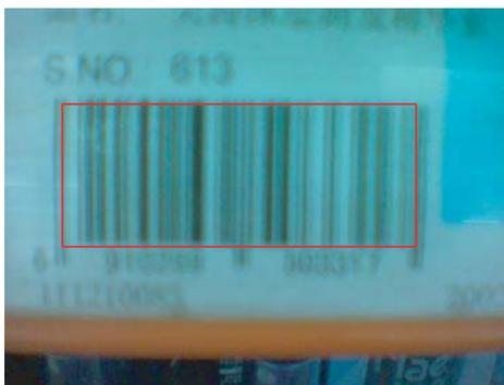
Fig. 6. The bar code area located.
