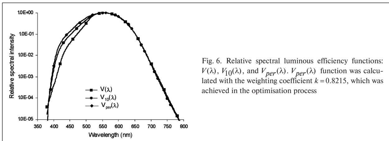
Fig. 6. Relative spectral luminous efficiency functions:  $V(\lambda)$ ,  $V_{10}(\lambda)$ , and  $V_{per}(\lambda)$ .  $V_{per}(\lambda)$  function was calculated with the weighting coefficient  $k = 0.8215$ , which was achieved in the optimisation process
