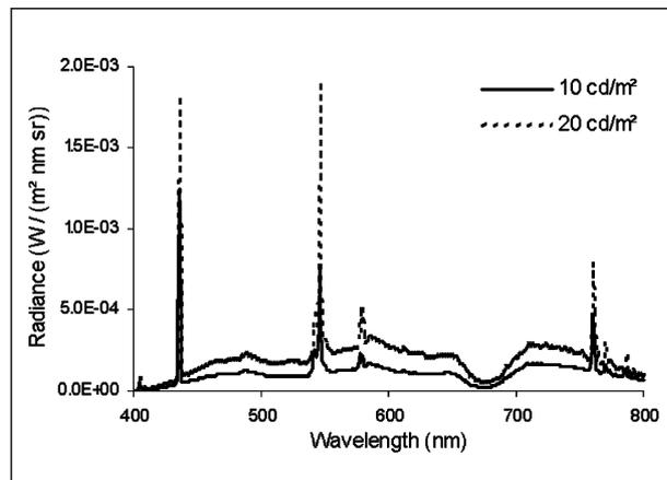
Fig. 1. The background of the hemisphere was illuminated with filtered 18 W fluorescent lamps with a CCT of 4930 K and 4610 K at 10 and 20  $\text{cd/m}^2$  background luminance, respectively
