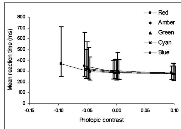
Fig. 3.  $RT$  as a function of stimulus spectra in foveal vision at  $10 \text{ cd/m}^2$ . The measurement points are the mean  $RT$ s of five subjects. In order to make the figure more clear, the contrasts of red and amber stimuli have been shifted by 0.005 and 0.0025 of the correct contrast, respectively, and cyan and blue stimuli by  $-0.0025$  and  $-0.005$ , respectively
