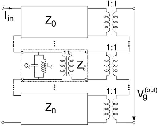
FIG. 5. Circuit network for pulse shaping by Cauer synthesis via the Laplace transform of the cosine Fourier series of Eq. (3), so  $Z_{12} = \sum_{\ell=0}^{\infty} a_{\nu}(\ell) (-1)^{\ell} s / [s^2 + (2\pi\ell/T)^2]$ .  $I_{in}$  is the input current pulse (here 55 ps) and  $V_g(s) = Z_{12}(s) I_{in}(s)$  relates to gate voltages  $n_{g\nu} = C_{G,\nu} v_{out,\nu} / 2e$  on qubits  $\nu=1, 2$ . All the values  $a_{\nu}(\ell)$ ,  $L_{\ell}$ , and  $C_{\ell}$  are tabulated in Table I.
