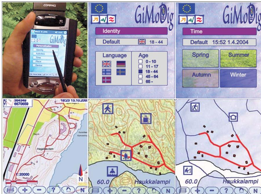
Figure 4. The GiMoDig- service delivers maps in real-time to the mobile devices. After personalisation of the service, the maps are automatically adapted to the different users in different usage situations.
