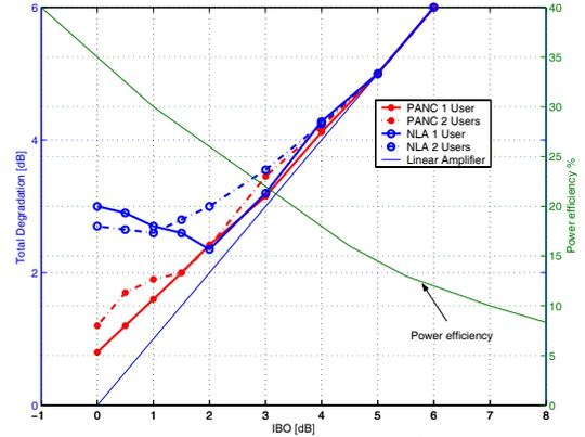
**Fig. 5.** Total Degradation as a function of back-off values
