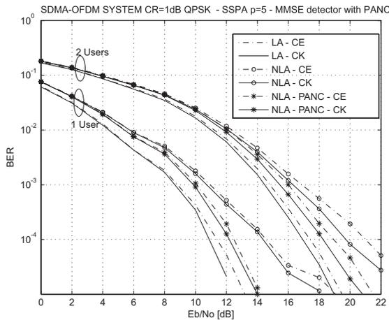
**Fig. 4.** BER SSPA with  $CR=1$  dB-MMSE receiver with PANC (CK-Perfect channel knowledge, CE-Channel estimation)
