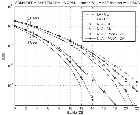
**Fig. 3.** BER Limiter with  $CR=1$  dB-MMSE receiver with PANC (CK-Perfect channel knowledge, CE-Channel estimation)
