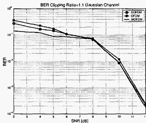
Fig. 6. BER with  $CR = 1.1$  and  $IBO = 0$  dB in AWGN Channel
