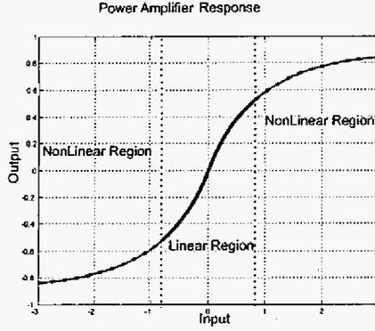
Fig. 1. Power Amplifier Response Characteristics
