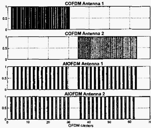
Fig. 4. Carrier allocation for COFDM and AIOFDM
