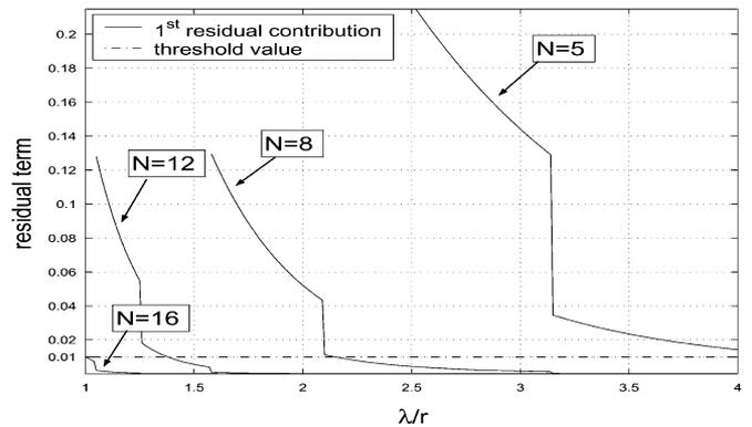
Fig. 6. Residual term as function of the UCA radius for different number of sensors. The residual value 0.01 is the threshold under which the residual error is considered to be negligible.
