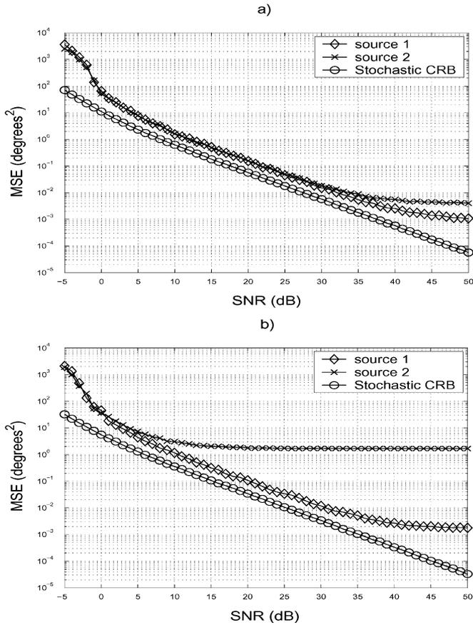
Fig. 10. Statistical performances of DoA algorithms for UCA when an (a) odd or (b) even small number of sensors is used. Bias appears as an error floor. Settings:  $N = 7$  in (a) and  $N = 8$  in (b) sensors,  $d = 0.3\lambda$ ,  $K = 500$ , and two uncorrelated sources located at  $(\phi_1, \phi_2) = (10^\circ, 25^\circ)$ .
