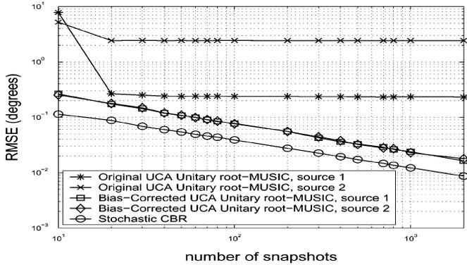
Fig. 15. Performances of the UCA unitary root-MUSIC algorithm. Settings:  $N = 8$ ,  $r = (\lambda/2.6)$ ,  $\text{SNR} = 50$  dB and  $(\phi_1, \phi_2) = (10^\circ, 15^\circ)$ .
