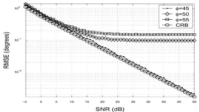
Fig. 9. Statistical performances of UCA unitary root-MUSIC algorithms for different source angles compared to the stochastic CRB. The bias in the DoA estimates clearly depends on the angle of arrival. Settings:  $N = 8$  sensors, interelement spacing  $d = 0.3\lambda$ , and  $K = 256$  snapshots.
