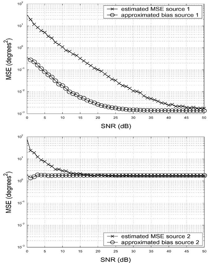
Fig. 5. Comparison between the estimated MSE of UCA unitary root-MUSIC and the first-order approximation of the squared bias term. For large values of SNR curves overlap. Settings:  $N = 8$ ,  $r = (\lambda/2.6)$ ,  $K = 500$ , two uncorrelated sources at  $(\phi_1, \phi_2) = (10^\circ, 25^\circ)$ , and 1000 independent Monte Carlo trials.
