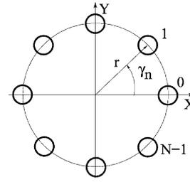
Fig. 2. UCA with  $N = 8$  sensors;  $r$  as the radius, and  $\gamma_n = (2\pi n)/(N)$  ( $n = 0, \dots, N-1$ ) as the angular position of a sensor.
