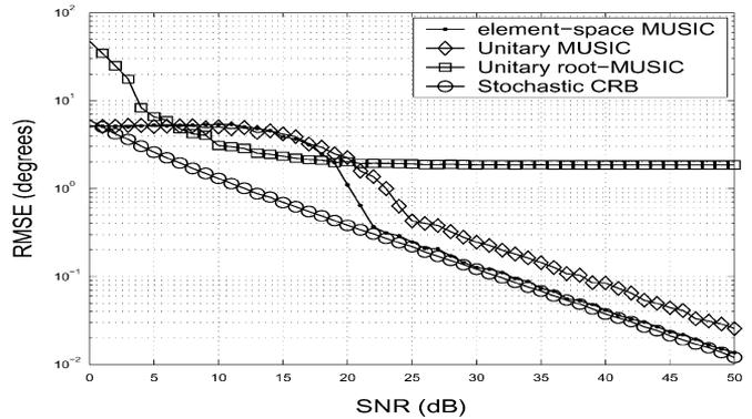
Fig. 8. RMSE of the DoA algorithms compared to CRB when a UCA with a small number of sensors is used. Only unitary root-MUSIC suffers from bias. Settings:  $N = 8$ ,  $r = (\lambda/2.6)$ ,  $d = 0.2944\lambda$ ,  $K = 256$  and the uncorrelated sources located at  $(\phi_1, \phi_2) = (10^\circ, 20^\circ)$ .
