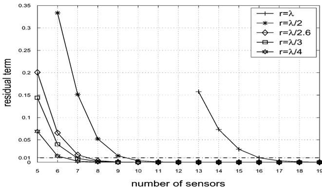
Fig. 7. Evaluation of the residual term. For fixed number of sensors the residual term grows as the UCA radius increases. For a fixed radius, however, it decreases as the number of sensors increases.
