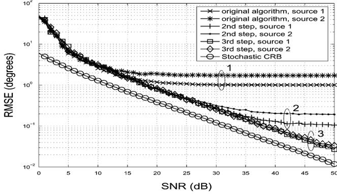
Fig. 14. Cancellation steps for the original UCA unitary root MUSIC algorithm, after the second iteration and after the third iteration. Settings:  $N = 8$ ,  $r = (\lambda/2.6)$ ,  $K = 256$ , and  $(\phi_1, \phi_2) = (15^\circ, 25^\circ)$ .
