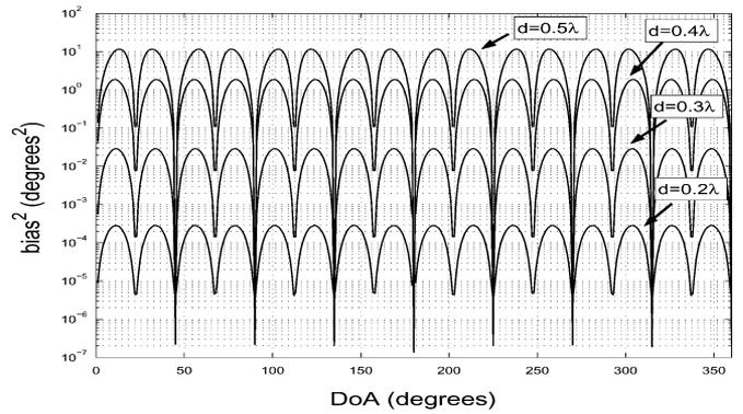
Fig. 12. Bias on the estimates of UCA unitary root-MUSIC as function of the DoAs for several interelement spacing  $d$  when  $N = 8$  sensors are used. Settings:  $K = 500$ ,  $\text{SNR} = 50$  dB. Note that the bias increases as the interelement spacing increases.
