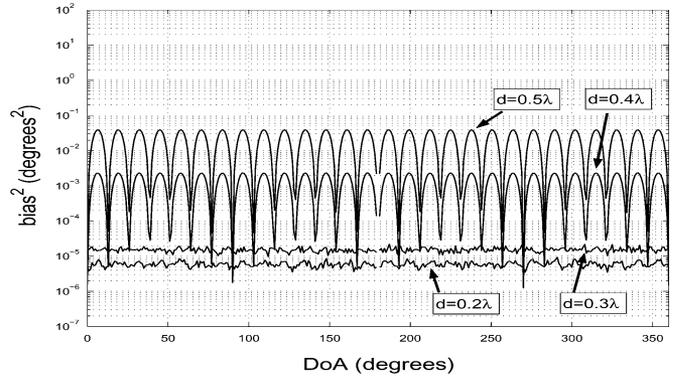
Fig. 13. Bias on the estimates of UCA unitary root-MUSIC as function of the DoAs when  $N = 7$  sensors are used. Settings:  $K = 500$ ,  $\text{SNR} = 50$  dB, and several interelement spacing  $d$ .
