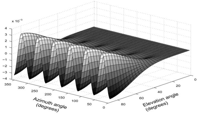
Fig. 3. Residual term as function of both azimuth  $\phi$  and elevation  $\theta$  angles. UCA settings:  $N = 8$ ,  $r = (\lambda/2.6)$  and  $f = 1.8$  GHz.
