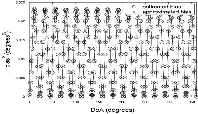
Fig. 4. Comparison between the estimated bias provided by UCA unitary root-MUSIC and the first-order approximation of the bias term. The approximation appears to be accurate since the curves overlap. The bias depends on the DoA.
