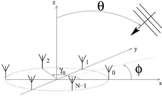
Fig. 1. UCA with  $N$  elements. The wavefield impinges to the array from a direction denoted by  $\theta$  (elevation) and  $\phi$  (azimuth). The array lies on the  $xy$  plane.
