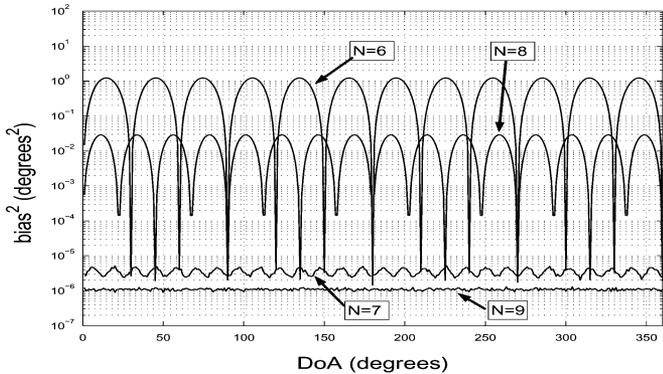
Fig. 11. Bias as function of the DoAs computed with UCA unitary root-MUSIC when different number of sensors are used. Settings:  $K = 500$ ,  $\text{SNR} = 50$  dB, and interelement spacing  $d = 0.3\lambda$ . Note that arrays with odd number of elements have lower bias.
