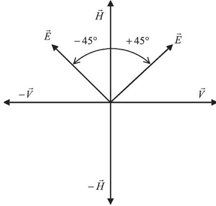
Fig. 1. Orientation of the measured electric field  $\vec{E}$  with respect to the polarization plane, defined by the vertical ( $\vec{V}$ ) and horizontal ( $\vec{H}$ ) polarizations, of the antenna of the radiometer in the setups of  $-45^\circ$  and  $+45^\circ$  angles.
