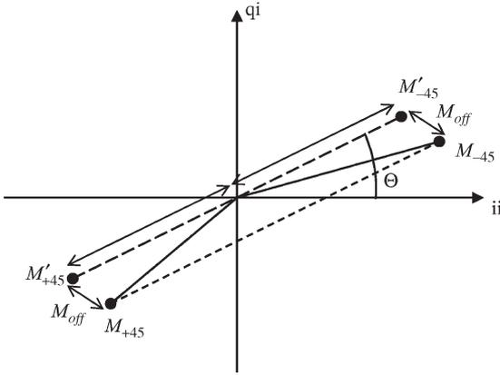
Fig. 2. Principle of the end-to-end phase difference retrieval. The offset remains the same in the two measurements, whereas the phase of the signal changes by  $180^\circ$ .  $M_{+45}$  and  $M_{-45}$  are the correlations measured at  $+45^\circ$  and  $-45^\circ$  angles,  $M_{\text{off}}$  is the offset of the measurement, and  $M'_{+45}$  and  $M'_{-45}$  are the correlations corrected with the offset.
