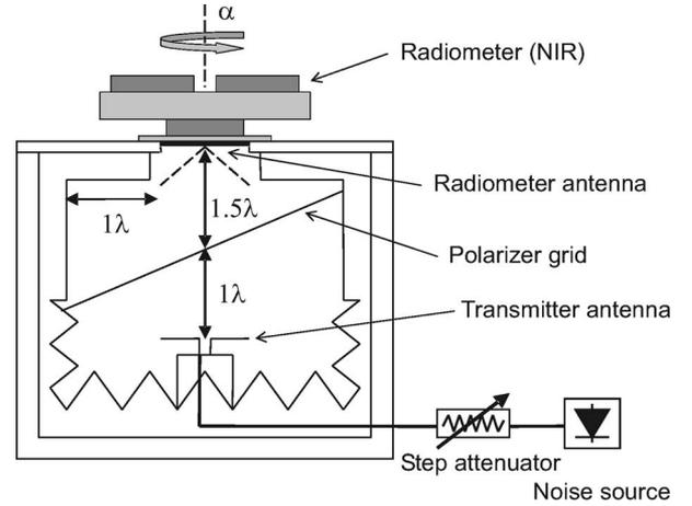
Fig. 3. Measurement setup utilizing the linearly polarized antenna target ( $\lambda$  stands for the free-space wavelength, which is 21 cm in this case).
