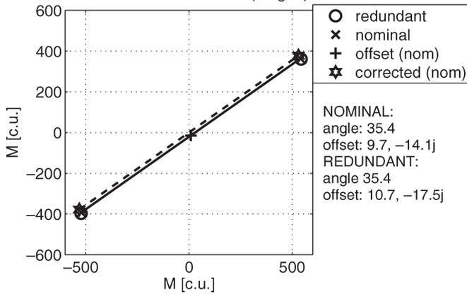
Fig. 6. Mean correlations at  $-45^\circ$  and  $+45^\circ$  rotation angles with the offset and the corrected values (for nominal correlations) when no grid was applied in the setup. The complex conjugate of the redundant correlation is taken before plotting.
