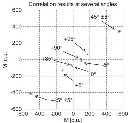
Fig. 4. Correlation results at rotation angles  $-45^\circ \pm 5^\circ$ ,  $0^\circ \pm 5^\circ$ ,  $+45^\circ \pm 5^\circ$ , and  $+90^\circ \pm 5^\circ$  for nominal and redundant correlations.
