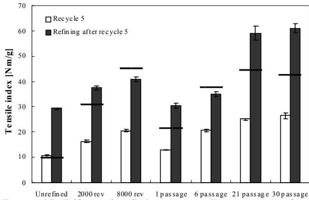
**Figure 10. Effect of refining on tensile strength of paper. Tensile strength for nonrecycled fibers is marked with a solid line. Error bars represent the 95% confidence interval.**
