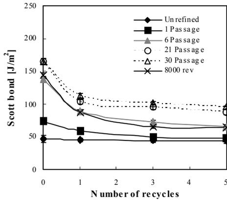
Figure 7. Effect of recycling on internal bond strength of paper. Error bars represent the 95% confidence interval.
