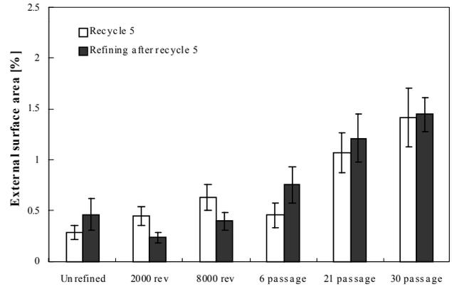
Figure 9. Effect of refining on external fibrillation. Error bars represent the 95% confidence interval.
