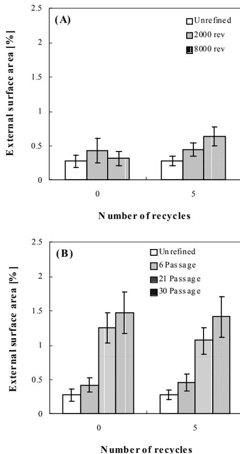
Figure 5. Effect of recycling on external fibrillation. Nonrecycled pulp was refined in the Lampén mill (A) and the grinder (B). Error bars represent the 95% confidence interval.
