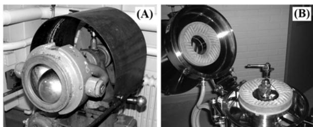
Figure 1. A Lampén mill (A) and an ultra-fine friction grinder [19] (B).
