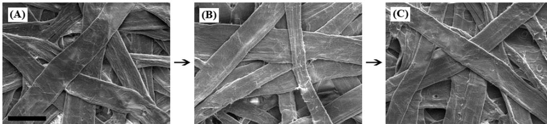
**Figure 12. SEM micrographs of a handsheet surface made from nonrecycled fibers (A), five-times recycled fibers (B) and five-times recycled, refined fibers (C). The pulp was refined to 8000 rev in the Lampén mill before recycling. Scale bar of 50  $\mu\text{m}$ .**
