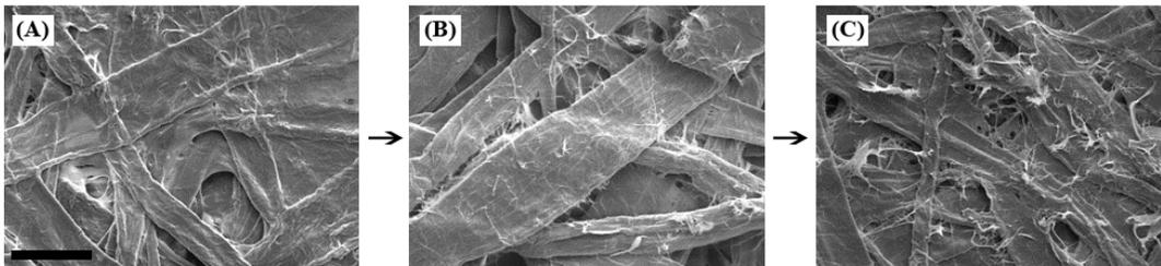
**Figure 13. SEM micrographs of a handsheet surface made from nonrecycled fibers (A), five-times recycled fibers (B) and five-times recycled, refined fibers (C). The pulp was recirculated 30 times in the grinder before recycling. Scale bar of 50  $\mu\text{m}$ .**
