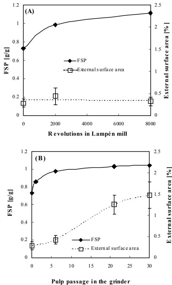
Figure 3. Development of internal and external fibrillation of fibers refined in the Lampén mill (A) and in the grinder (B). Pulp passage is defined as the number of times that the pulp is recirculated through the gap in the grinder. Error bars represent the 95% confidence interval, otherwise the average of two measurements is shown.
