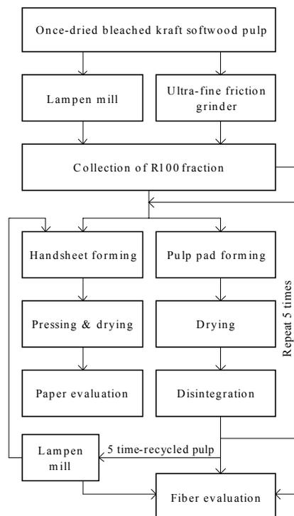
Figure 2. Procedure for recycling experiment.
