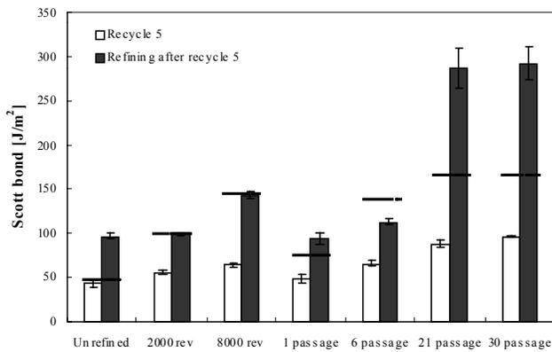
**Figure 11. Effect of refining on internal bond strength of paper. Internal bond strength for nonrecycled fibers is marked with a solid line. Error bars represent the 95% confidence interval.**
