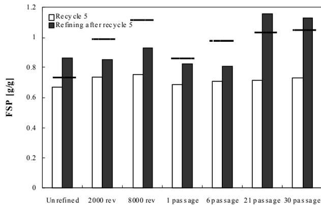
Figure 8. Effect of refining on internal fibrillation. The FSP for nonrecycled fibers is marked with a solid line.
