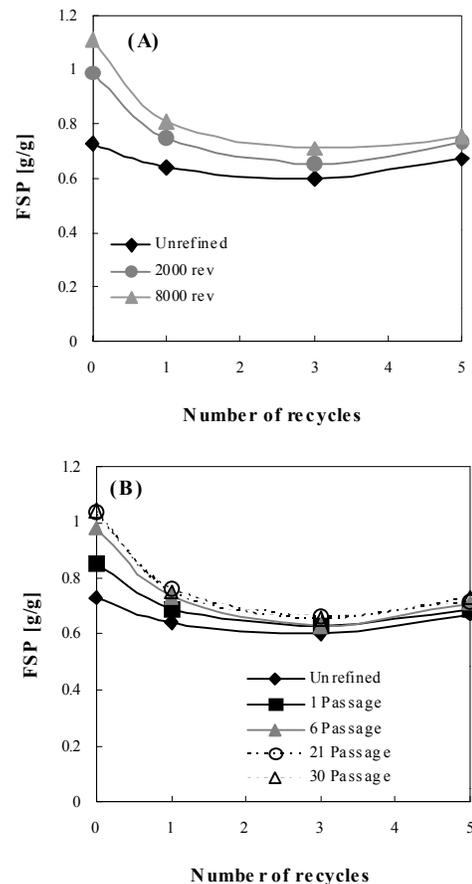
Figure 4. Effect of recycling on internal fibrillation. Nonrecycled pulp was refined in the Lampén mill (A) and the grinder (B).
