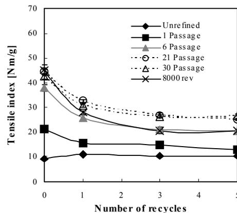
Figure 6. Effect of recycling on tensile strength of paper. Error bars represent the 95% confidence interval.
