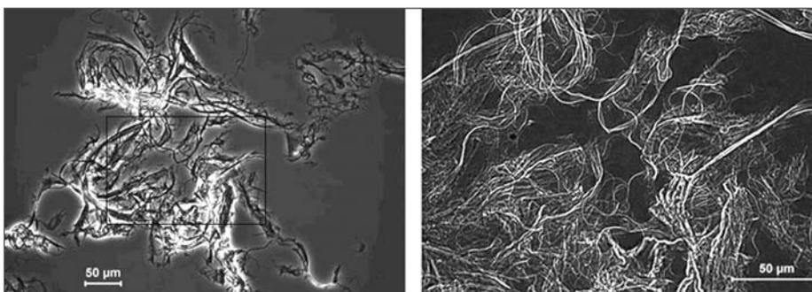
2. Microscopic images of fines (P100 fraction), 60 μm-7P. Phase contrast mode (left) and bright field with polarized light mode (right).
