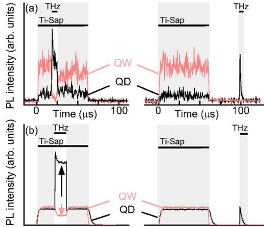
FIG. 8. (Color online) Experimental (a) and simulated (b) time-resolved PL of the QD ground state (black) and QW (red) for  $T = 15$  K. The energy and power of the THz radiation were  $\hbar\omega_{\text{THz}} = 2.5$  meV and  $P = 1$  kW, respectively. The time windows of the Ti-Sap laser (carrier generation to the QW) and THz-radiation are indicated by horizontal bars.
