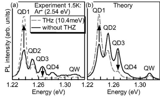
FIG. 7. Experimental (a) and theoretical (b) photoluminescence from a sample pumped by an Ar<sup>+</sup> laser only (solid lines) and by Ar<sup>+</sup> laser and FEL simultaneously (dashed line). The FEL energy of the experiments was  $\hbar\omega_{\text{THz}} = 10.4$  meV.
