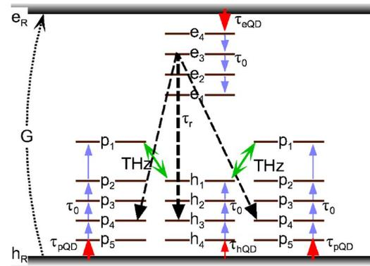
FIG. 6. (Color online) Carrier dynamics model. The eigenstates of the DP minima are labeled  $e_i$  and  $h_i$ ; the hole states of the PEP minima are labeled  $p_i$ . The pump laser  $G$  generates carriers to the reservoirs ( $e_R$  and  $h_R$ ) and the resonant THz radiation transfers holes between the ground states  $p_1$  and  $h_1$ . Radiative recombinations (black dashed arrows) are shown for the third electron level only. The energy scale is only schematic.
