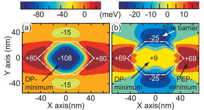
FIG. 2. (Color online) Potential energy of (a) electrons and (b) holes, in the middle of the QW (8.25 nm below the InP island). The energies are given with respect to the band edges of an  $\text{In}_{0.2}\text{Ga}_{0.8}\text{As}$  QW, far away from the island. The white dashed lines show the bottom contour of the InP island and the labels correspond to the local potential maxima/minima.
