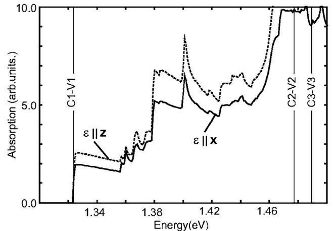
FIG. 9. Absorption coefficient for the strained CC structure of Fig. 1(b). The solid and dotted lines correspond to the absorption of light polarized in  $x$  and  $z$  directions, respectively ( $z$  is parallel to the QWRS). The absorption coefficient was calculated without any linewidth broadening in order not to smear out the fine structure. The vertical lines indicate the energies of the diagonal transitions at  $\mathbf{k}=0$ .
