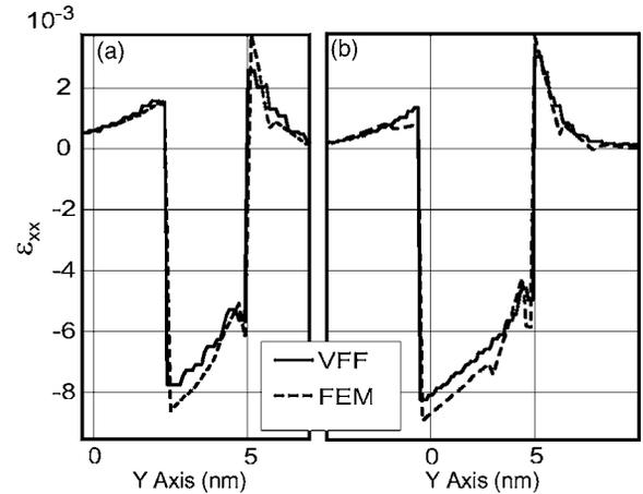
FIG. 2. The strain component  $\epsilon_{xx}$  in the crystal coordinate system along the vertical line shown in Fig. 3. In (a) the thickness is  $T_{QW}=3$  nm, and in (b)  $T_{QW}=6$  nm. The VFF and FEM results are shown by solid and dashed lines, respectively.
