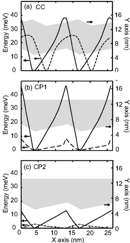
FIG. 10. Effective potential energy of an electron (solid line) and a hole (dashed line) as a function of  $x$  coordinate, in (a) the strained CC, (b) the strained CP1, and (c) the lattice-matched CP2 structure. The shaded areas and the  $y$  axis to the right show the corresponding geometry.
