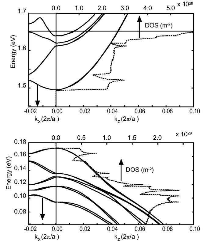
FIG. 6. The band diagram (solid lines) and DOS (dotted lines) for the strained CC structure. The band energy is given with respect to the strain-free valence band edge of bulk  $\text{Al}_{0.2}\text{Ga}_{0.8}\text{As}$ . The axis below the panels correspond to the wave vector of the energy bands and the axis at the top correspond to the DOS. The energy scale to the left is common to all curves.
