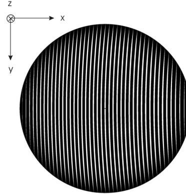
Figure 2: An example of hologram pattern used in CATR. Slots are in white, metal stripes in black.
