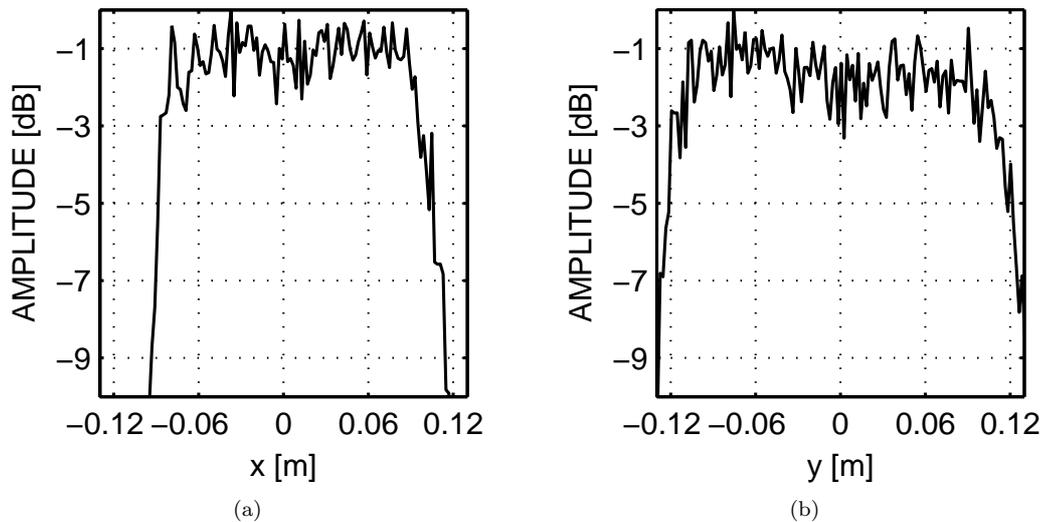
Figure 5: Measured amplitude of the quiet-zone field at 0.9 m from the hologram: (a) along a horizontal cut  $y = 0$ , (b) along a vertical cut  $x = 0$ .
