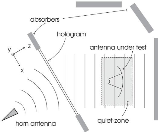
Figure 1: A schematic layout of hologram based CATR.
