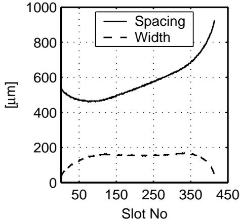
Figure 3: Widths and spacings of slots along the horizontal center line of the hologram.
