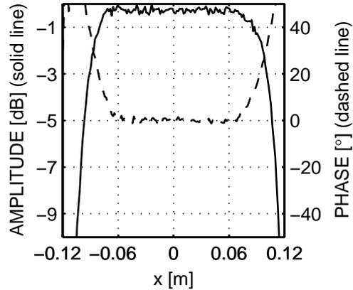
Figure 4: Horizontal cut ( $y = 0$ ) of simulated quiet-zone field at 0.9 m from the hologram.
