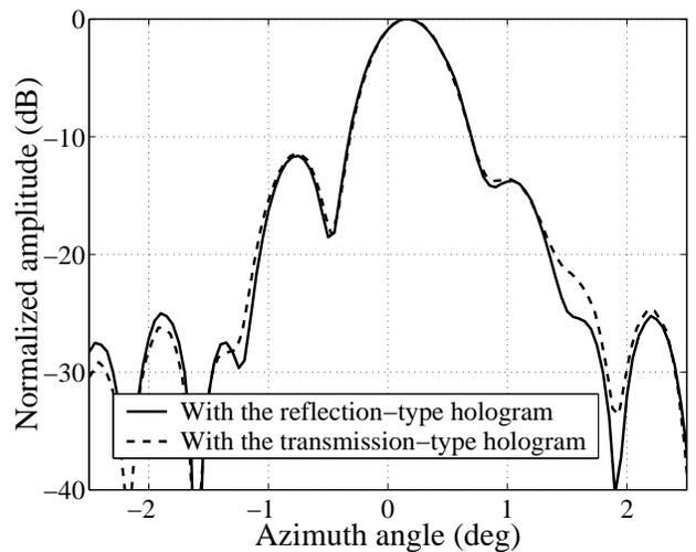
Figure 7. Close-up of the antenna main beam.
