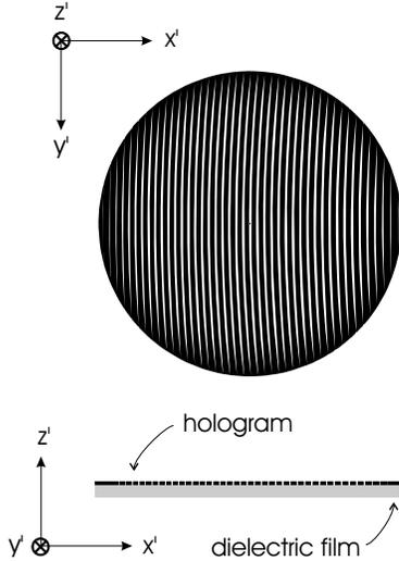
**Figure 1. An amplitude hologram. Slots are in white, metal strips in black.**
