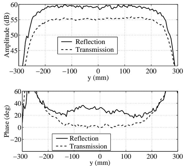
**Figure 5. Measured vertical cut of the quiet-zone for the reflection- and transmission-type holograms.**
