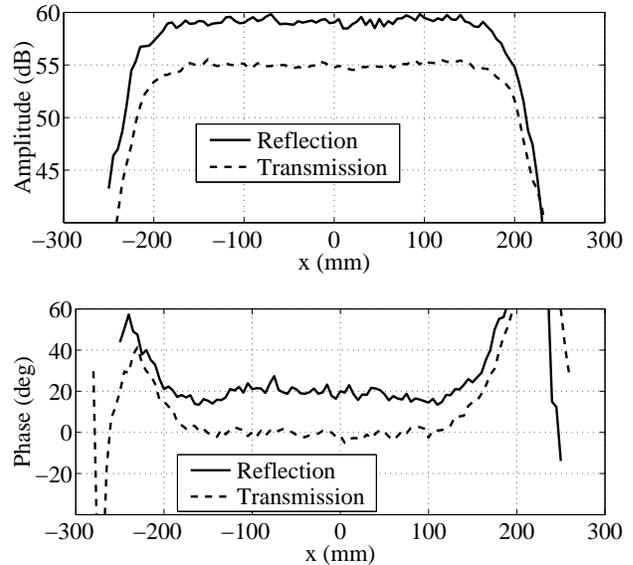
**Figure 4. Measured horizontal cut of the quiet-zone for the reflection- and transmission-type holograms.**
