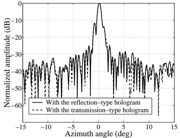
Figure 6. Antenna radiation pattern in the azimuth plane at 310 GHz measured with the reflection- and transmission-type holograms.
