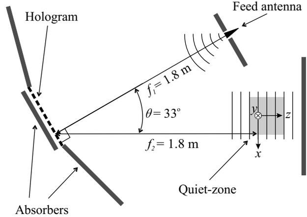
**Figure 2. The CATR based on the reflection-type hologram studied in this paper.**
