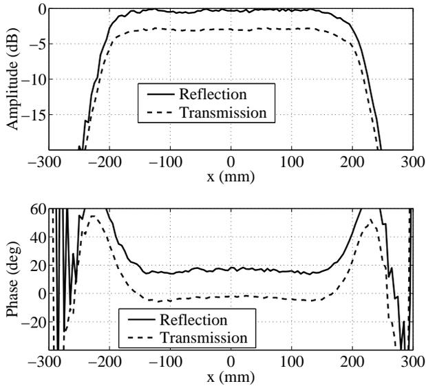
**Figure 3. Simulated horizontal cut of the quiet-zone for the reflection- and transmission-type holograms.**
