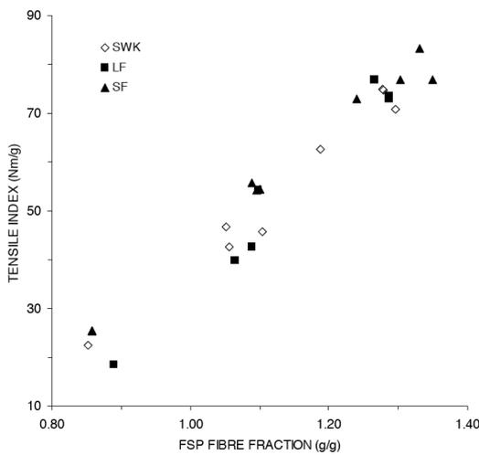
Fig 4. Effect of FSP on tensile strength.
