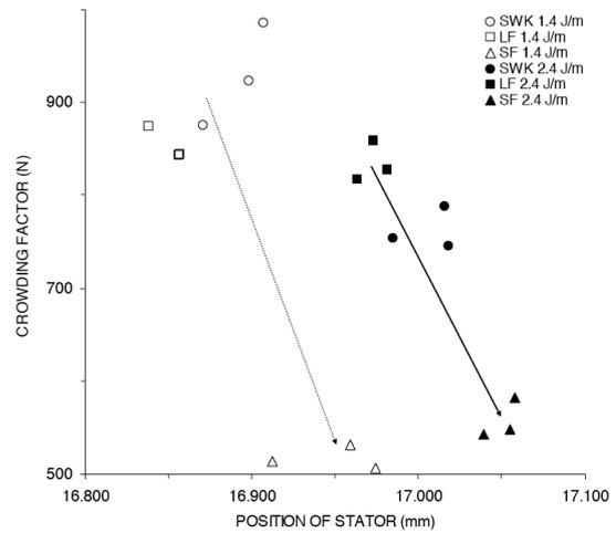
Fig 1. Crowding factor versus position of stator at refining intensities of 1.4 and 2.4 J/m.
