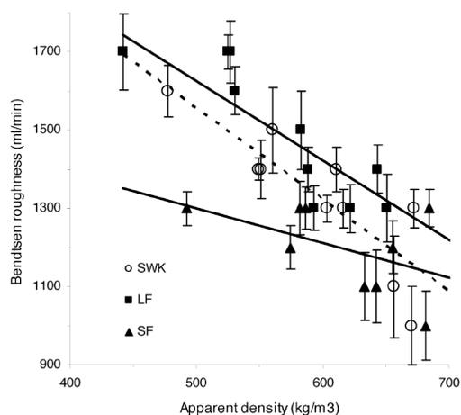
Fig 6. Characteristics of density-Bendtsen roughness combination of fractions.
