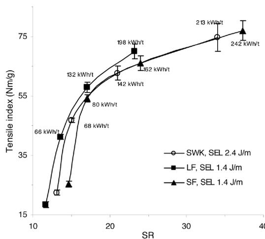
Fig 5. Characteristics of dewatering resistance (SR) - tensile index combination. The best intensity for the specific fraction was selected.
