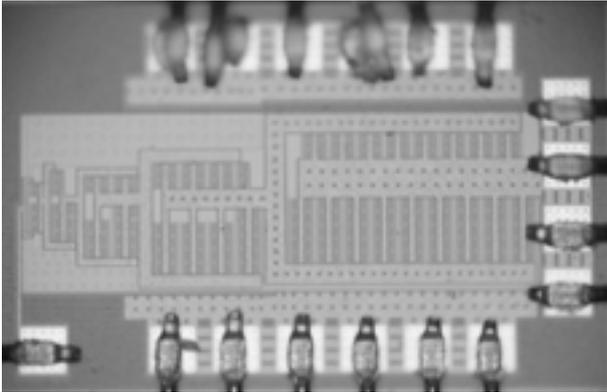
**Figure 5.** Microphotograph of the push-pull amplifier chip
