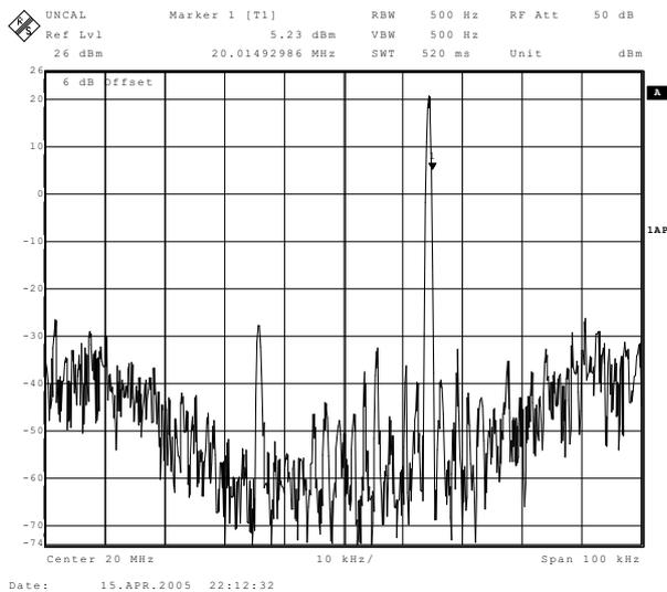
**Figure 7.** Measured inband spectrum from the Class-D amplifier driven with a BP-PWM signal
