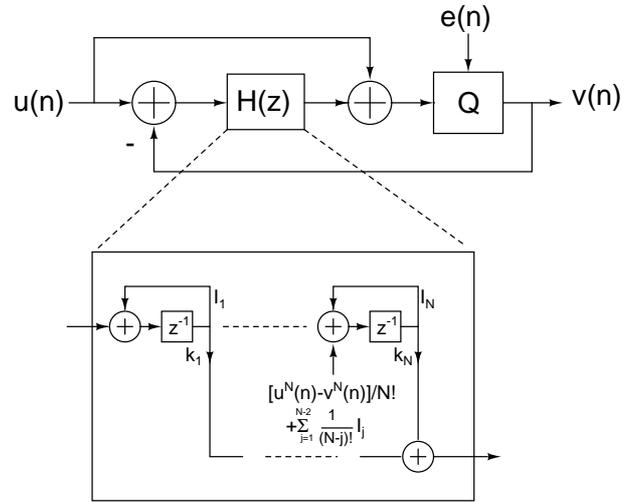
Figure 3. Integral noise shaping block diagram (INS in Fig. 2)
