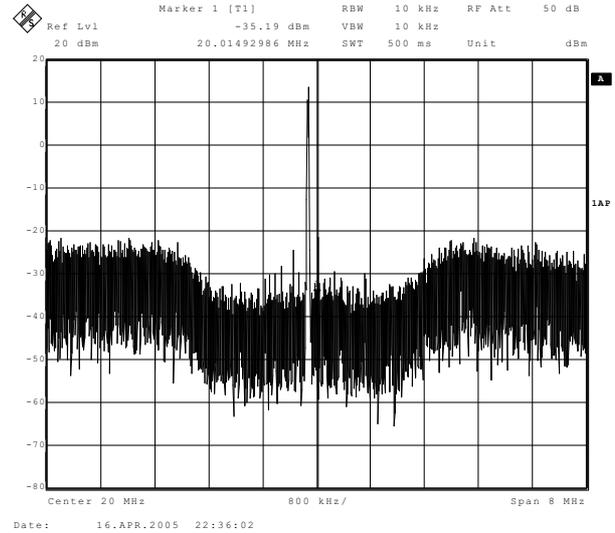
**Figure 6.** Measured inband spectrum from the Class-D amplifier driven with a bandpass  $\Delta\Sigma$ -modulated signal
