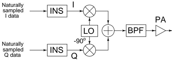
Figure 2. Bandpass pulse width modulation using digital quadrature modulation
