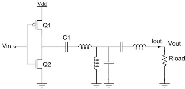
**Figure 4.** Voltage mode class-D power amplifier
