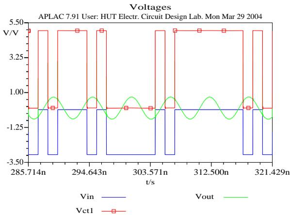
Figure 7. Voltages in a H-bridge VMCD amplifier.
