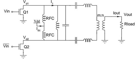
Figure 5. A circuit-model of a current-mode class-D amplifier
