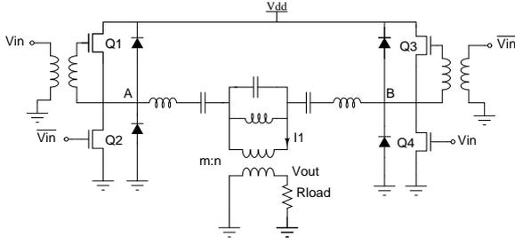
Figure 2. An H-bridge voltage-mode Class-D amplifier
