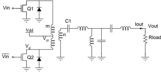
Figure 3. A transformer-coupled voltage-mode class-D amplifier
