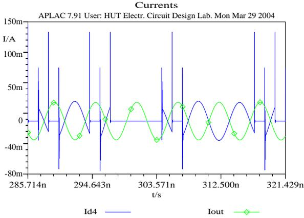
Figure 6. Currents in a H-bridge VMCD amplifier.
