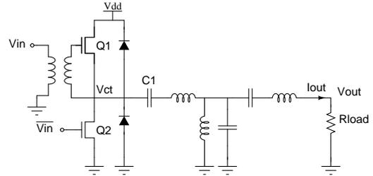
Figure 1. A schematic of a voltage mode class-D amplifier
