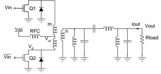
Figure 4. A transformer-coupled current-mode class-D amplifier
