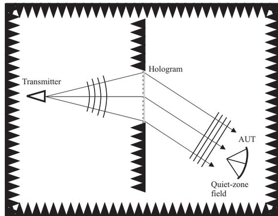
Figure 1. Geometry of a CATR based on a transmission-type hologram.
