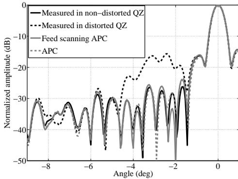
Figure 4. The antenna patterns with the feed scanning APC.
