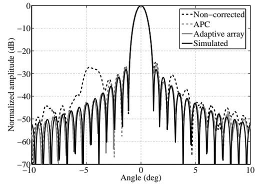
Figure 6. The antenna patterns with the adaptive array correction.
