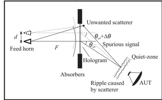
Figure 2. The phase of the direct signal and spurious signal changes differently when the range feed is displaced.
