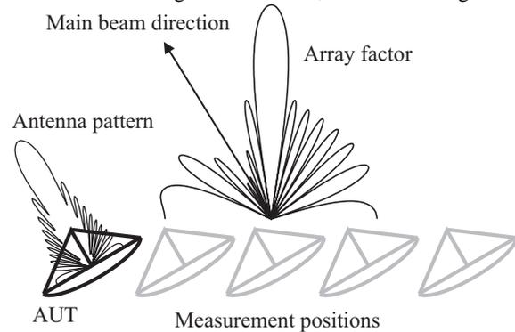
Figure 3. A virtual antenna array is formed, when the antenna pattern of the AUT is measured at different locations in the quiet-zone.
