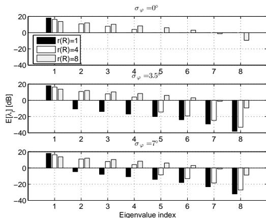
Fig. 2. Spectrum of  $8 \times 8$  MIMO physical channel correlation matrix with different ranks subject to PN impact.
