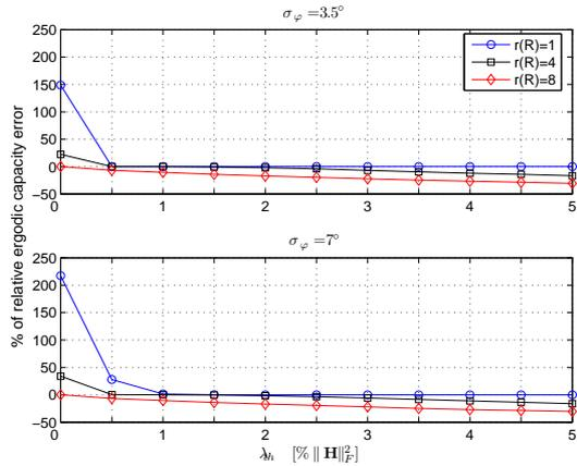
Fig. 3. Percentage of relative ergodic capacity error with EVF at different threshold of  $8 \times 8$  MIMO system subject to PN.
