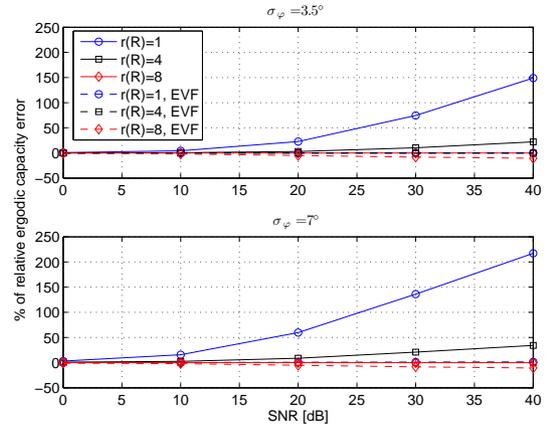
Fig. 4. Percentage of relative ergodic capacity error without and with EVF  $\lambda_{th} = 0.01 \|\mathbf{H}\|_F^2$  of  $8 \times 8$  MIMO system.
