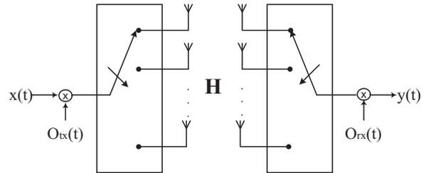
Fig. 1. Sketch of a TDMS based MIMO channel sounder.
