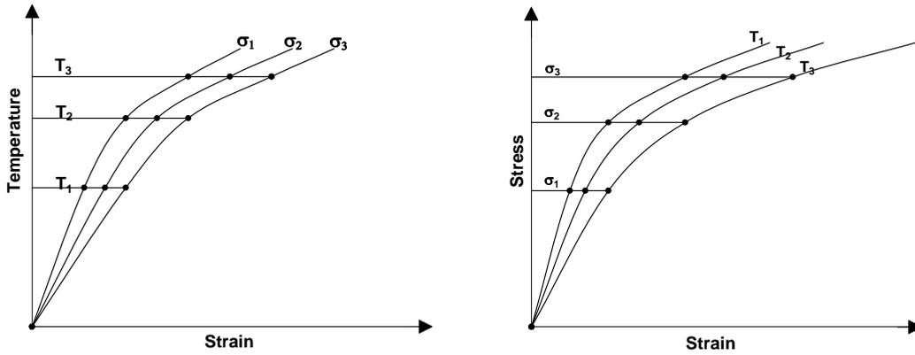
**Figure 3:** Converting the stress-strain curves from the transient state test results.
