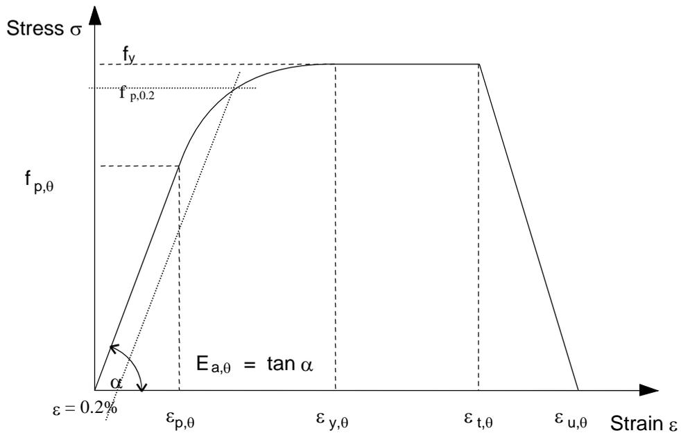
**Figure 4:** Stress-strain relationship for steel at elevated temperatures.
