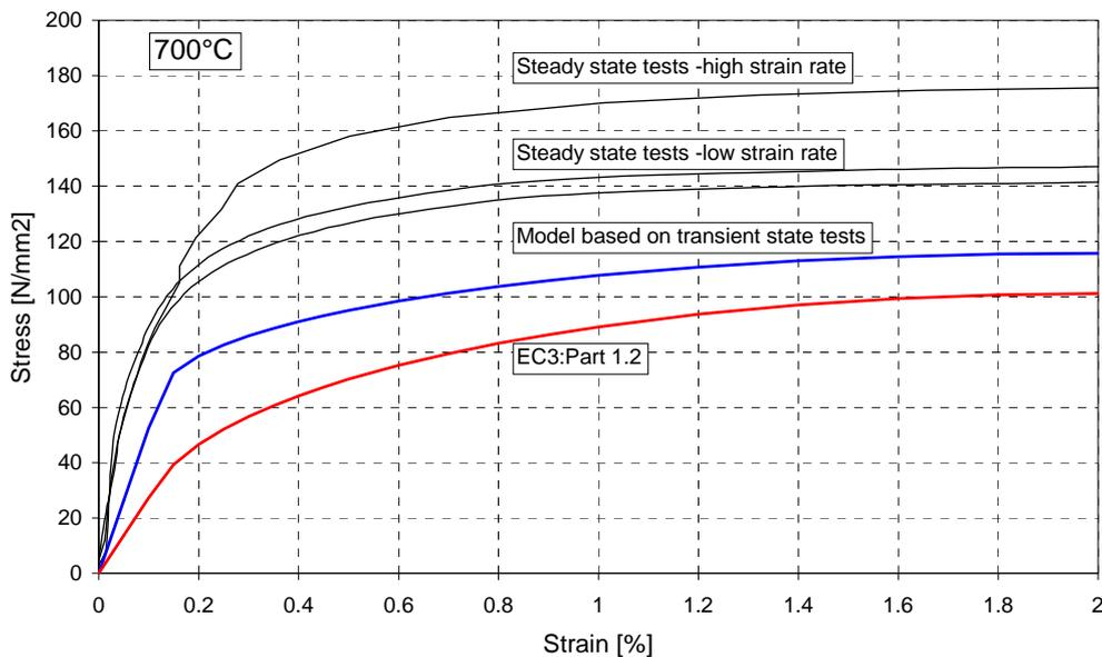
**Figure 14:** Effect of strain rate on test results of structural steel S460.
