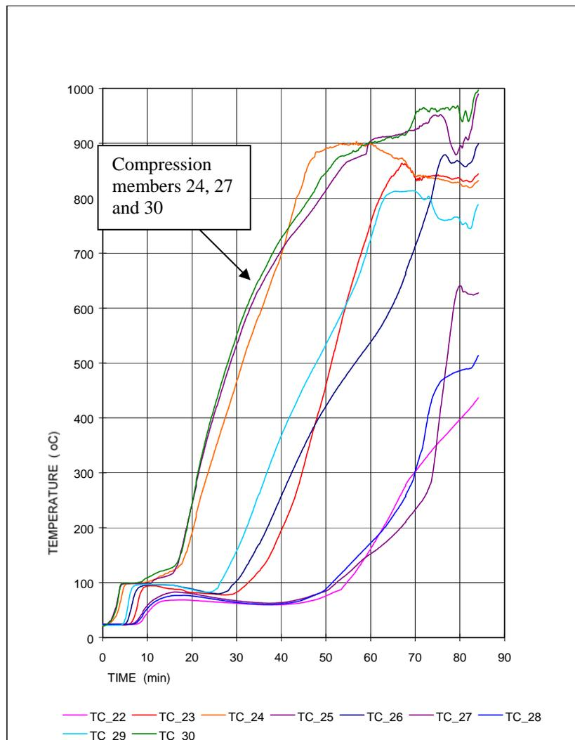
**Figure 16:** Temperature histories of the compression test specimens, from which the tensile test specimens were taken after cooling down.
