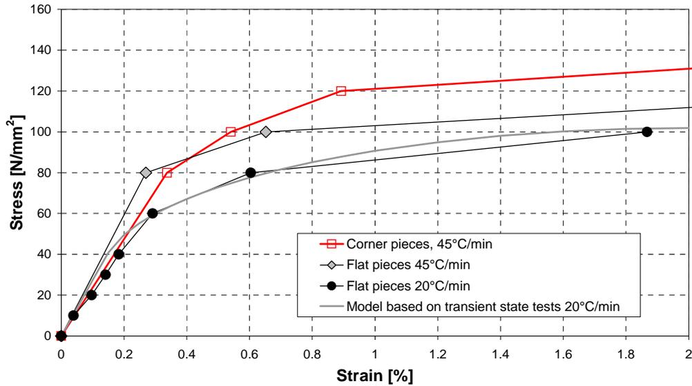
**Figure 13:** Stress-strain curves of structural steel S355J2H. Test results with different specimens and different heating rates at temperature 700 °C.
