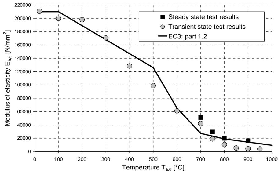
**Figure 12:** Modulus of elasticity of structural steel S355 at elevated temperatures (App. A).
