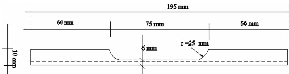
Test piece 4 (corner part from different sized RHS tubes (manufacturer Rautaruukki)).
