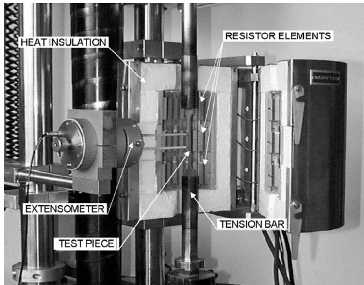
**Figure 1:** High-temperature tensile testing device.
