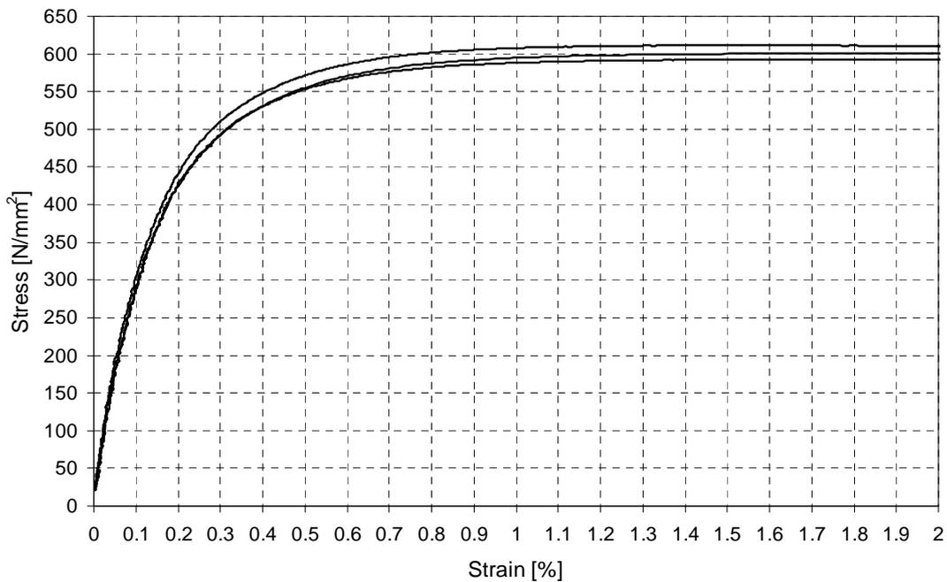
**Figure 10:** Tensile test results at room temperature for structural steel S355J2H. Test pieces taken from the corner part of SHS 50x50x3.
