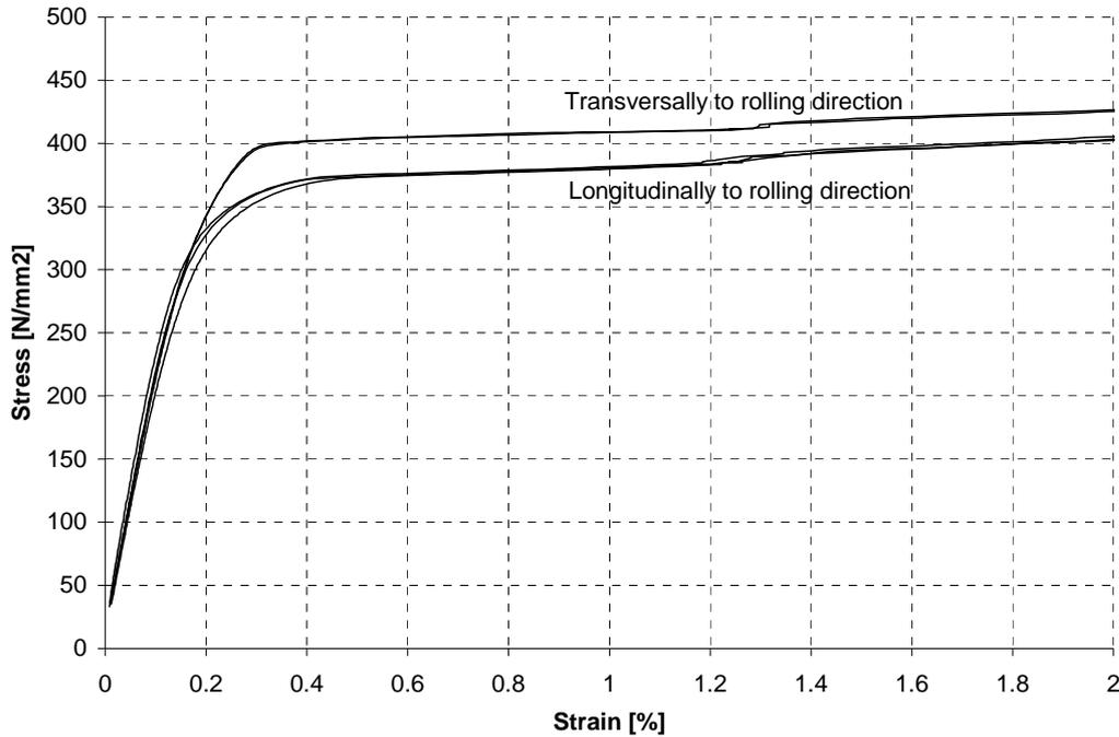
**Figure 8:** Stress-strain curves for structural steel S350GD+Z at room temperature.
