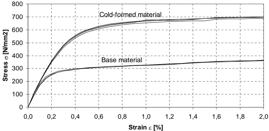
**Figure 5:** Stress-strain curves of stainless steel EN 1.4301 at room temperature.
