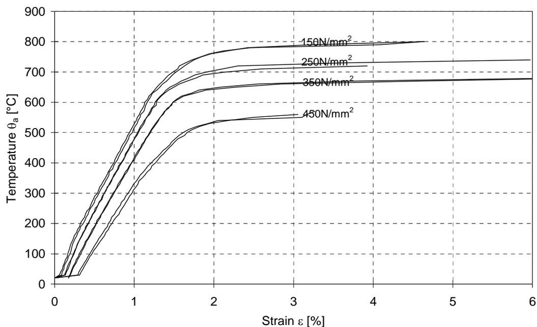
**Figure 11:** Temperature-strain curves from the transient state tests of austenitic stainless steel EN 1.4301 (App. C).
