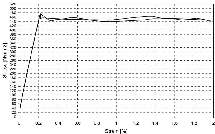
Figure 7: Stress-strain curves from tensile tests at temperature 20 °C for structural steel S460M.
