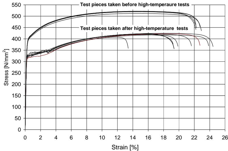
**Figure 17:** Tensile test results for structural steel S350GD+Z. Test pieces taken before and after high-temperature compression tests.
