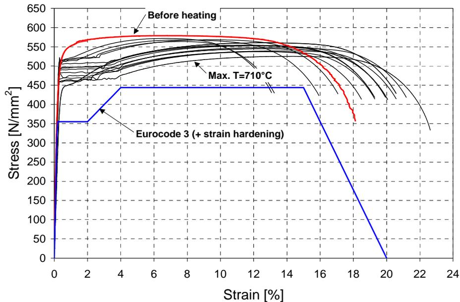
**Figure 15:** Tensile test results of structural steel S355J2H.
