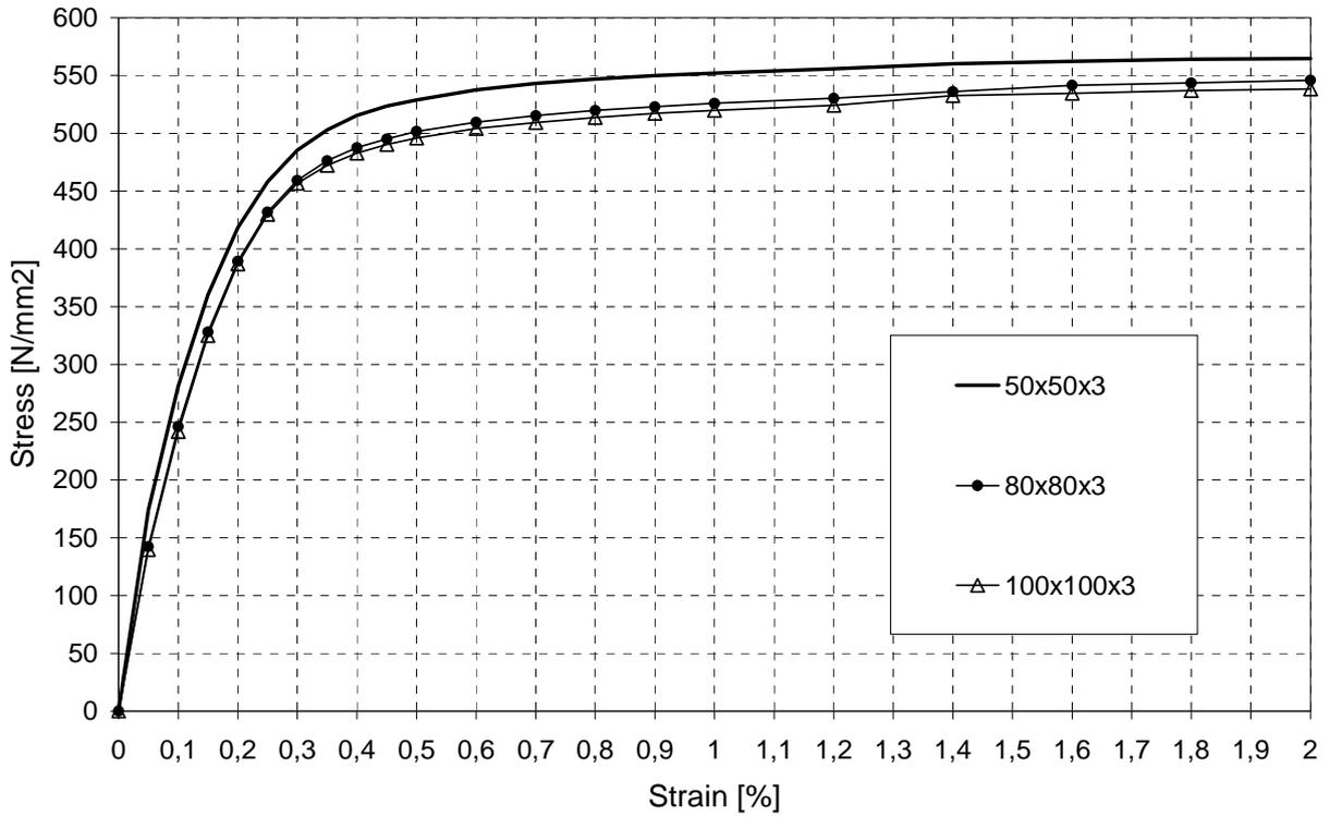
**Figure 9:** Tensile test results at room temperature for structural steel S355J2H. Test pieces taken from SHS 50x50x3, 80x80x3 and 100x100x3.
