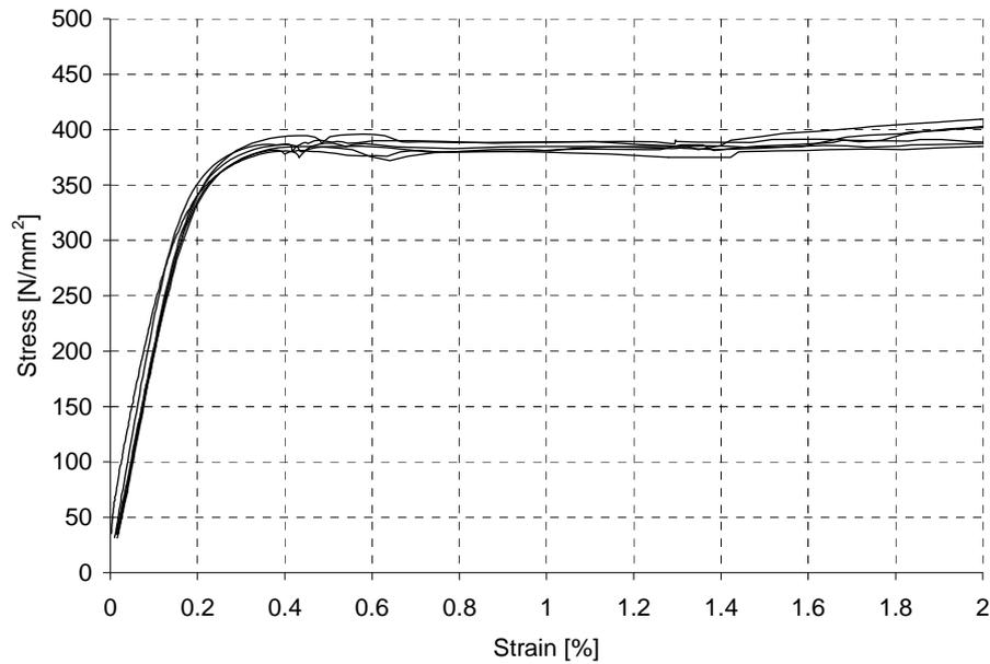
**Figure 6:** Stress-strain curves of structural steel S355 at room temperature.
