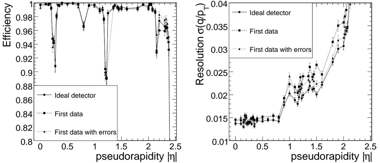
Figure 2: Muon reconstruction efficiency (left) and  $1/p_T$  resolution (right) as a function of the pseudorapidity  $\eta$  for muons with the generated  $p_T$  of 100 GeV, for the ideal alignment and for the *First Data* scenario with and without the muon APE. The nominal geometry of the tracker is used in all three cases.
