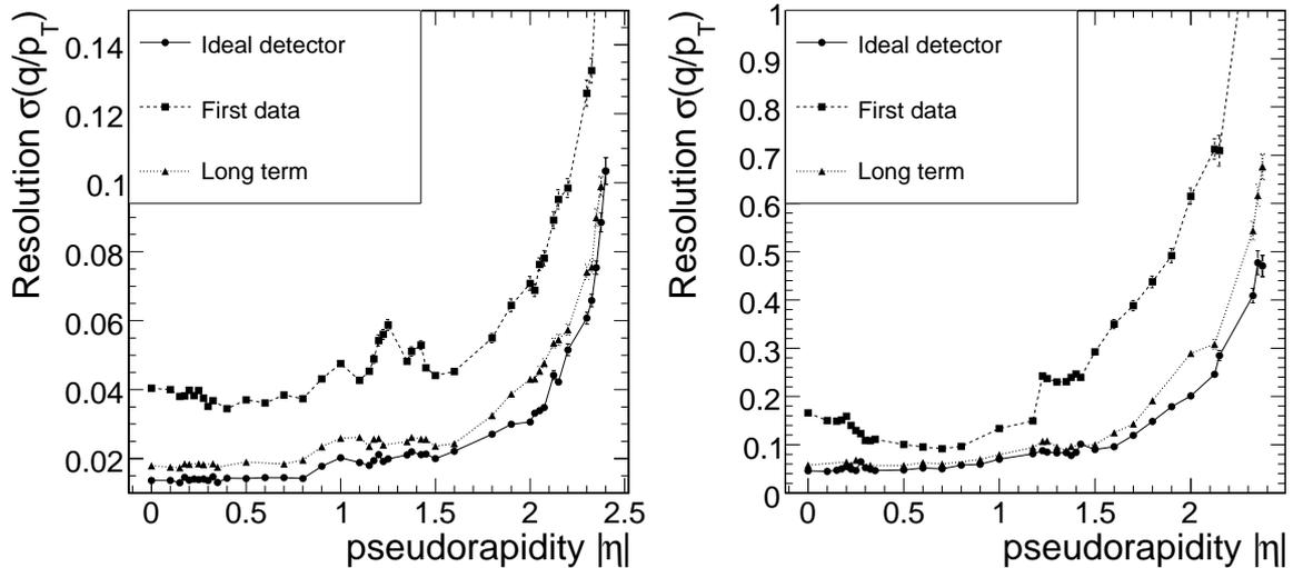
Figure 5: Muon  $1/p_T$  resolution (sigma of a Gaussian fit) as a function of  $\eta$  for the ideal alignment and for the *First Data* and *Long Term* scenarios applied simultaneously to the Tracker and to the muon detector, for  $p_T^{\text{gen}} = 100 \text{ GeV}$  (left) and  $p_T^{\text{gen}} = 1 \text{ TeV}$  (right).
