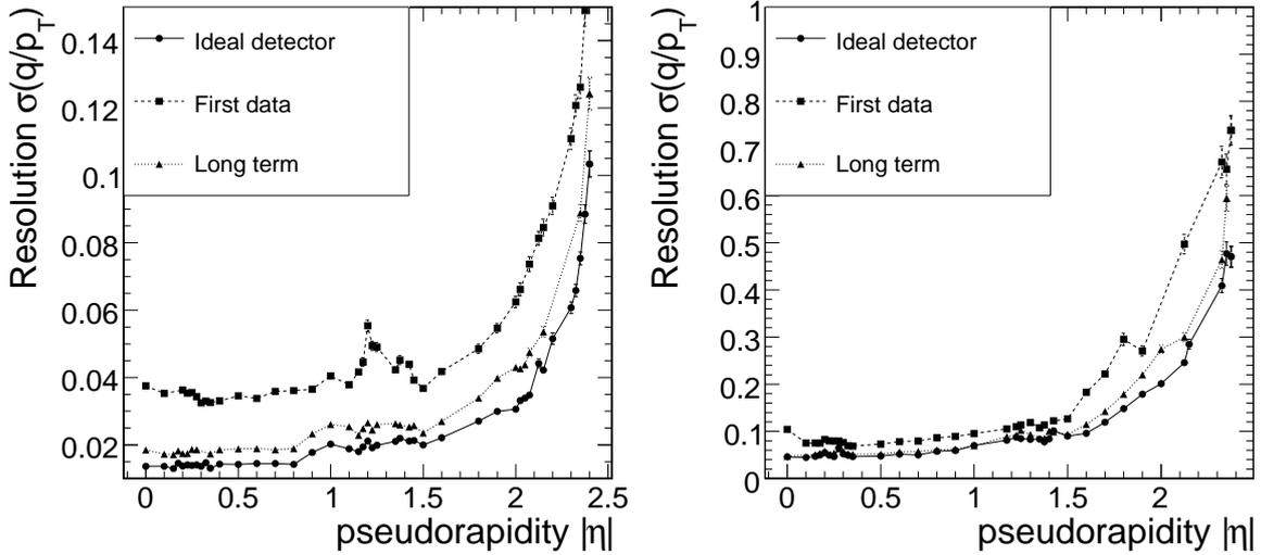
Figure 3: Muon  $1/p_T$  resolution (sigma of a Gaussian fit) as a function of  $\eta$  for the ideal alignment and for the *First Data* and *Long Term* Tracker misalignment scenarios, for  $p_T^{\text{gen}} = 100$  GeV (left) and  $p_T^{\text{gen}} = 1$  TeV (right).
