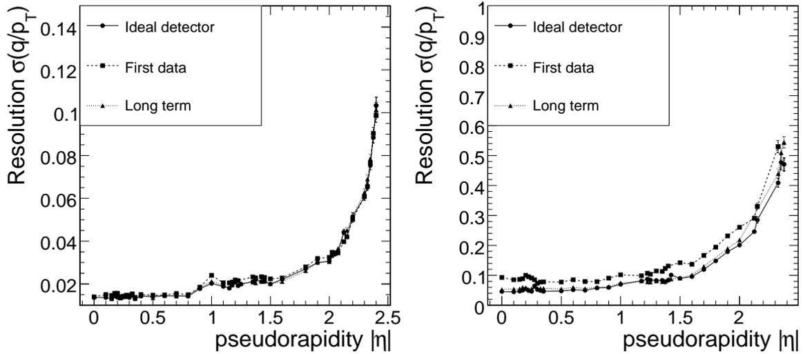
Figure 4: Muon  $1/p_T$  resolution (sigma of a Gaussian fit) as a function of  $\eta$  for the ideal alignment and for the *First Data* and *Long Term* muon misalignment scenarios, for  $p_T^{\text{gen}} = 100 \text{ GeV}$  (left) and  $p_T^{\text{gen}} = 1 \text{ TeV}$  (right).
