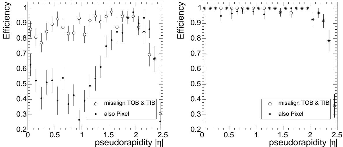
Figure 1: Track-finding efficiency as a function of the pseudorapidity  $\eta$ , for misaligned TOB and TIB (open circles), and for misaligned TOB, TIB and the Pixel detector (dark circles). Left: the APE is not taken into account; Right: the APE is taken into account.
