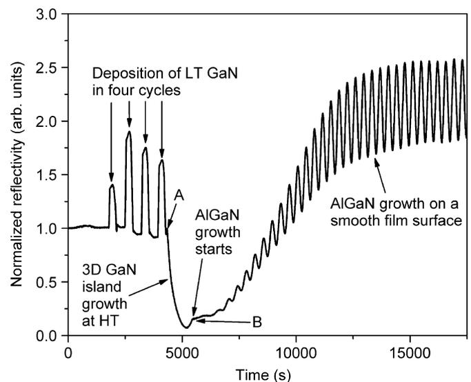
Fig. 1. In situ reflectivity data from the multistep AlGa<sub>0.12</sub>N process. Critical points in the process are labeled in the graph.
