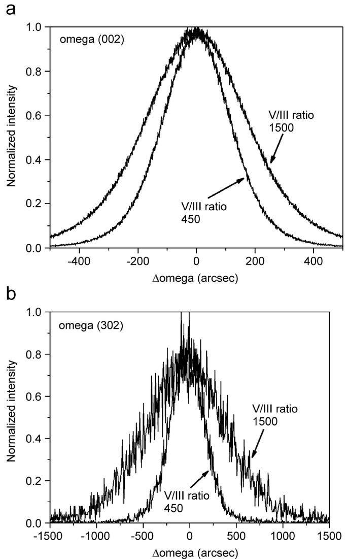
Fig. 5. HR-XRD data from the (a) (002) and (b) (302) diffraction of AlGa<sub>N</sub>. The data were recorded in a rocking curve scan for the two  $\text{Al}_{0.12}\text{Ga}_{0.88}\text{N}$  layers in Fig. 4.
