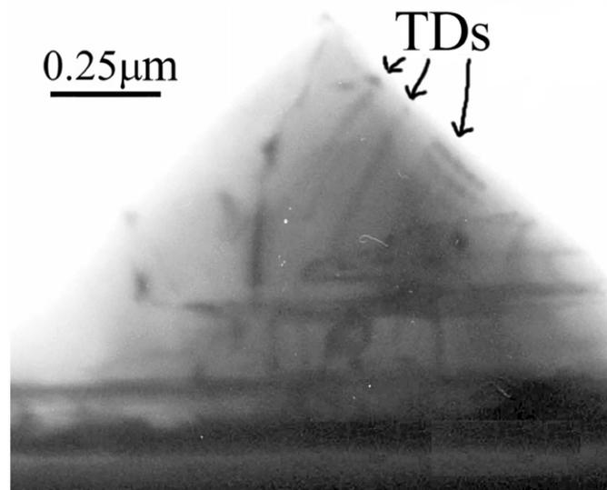
Fig. 3. Cross sectional TEM data presenting the TD content in a GaN NI. The NI was grown with a small V/III ratio of 450 to stimulate TD inclination towards the high index facets of the island.
