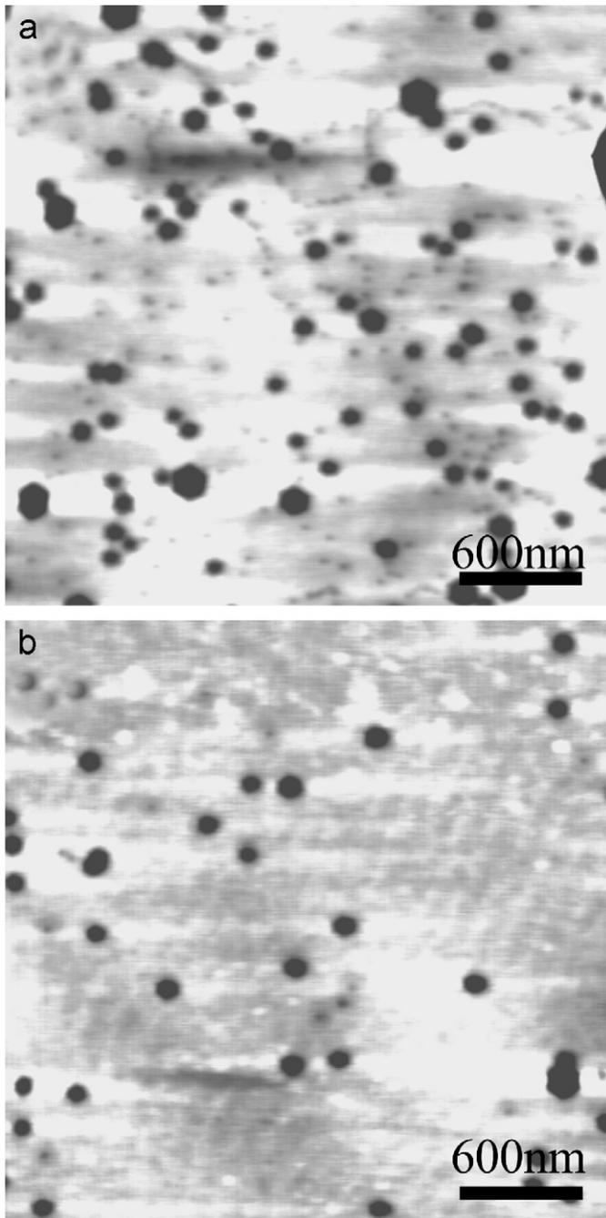
Fig. 4. Etch-pit density data obtained by AFM. A V/III ratio of 1500 (a) and 450 (b) were used during the HT GaN growth to affect the shape of the nucleation islands. A TD density of  $2.8 \times 10^9$  and  $5 \times 10^8 \text{ cm}^{-2}$  can be calculated for the two samples, respectively. The scale of the images is  $3 \times 3 \mu\text{m}$ .
