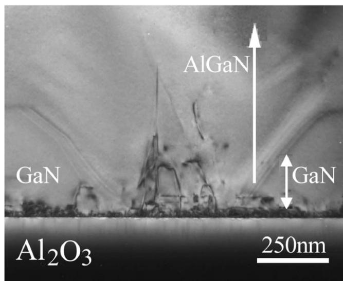
Fig. 6. Cross sectional TEM data presenting TDs generated at the exposed areas of the sapphire interfacial layer in between two GaN NIs. The data were taken from sample A.
