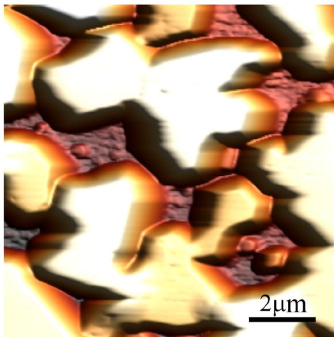
Fig. 2. AFM data illustrating the surface morphology of the GaN NL in the multistep AlGaN process prior to the beginning of AlGaN growth. The scale of the image is  $10 \times 10 \mu\text{m}$ .
