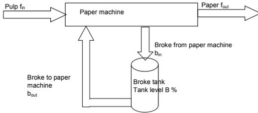
Figure 11. Simplified paper machine broke system
