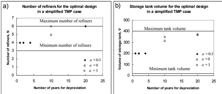
Figure 8. Risk premium weighting effect ( $a = 0$  to  $3$ ) on the optimal design in the simplified TMP case with different number of years for depreciation: (a) number of refiners and (b) storage tank volume.
