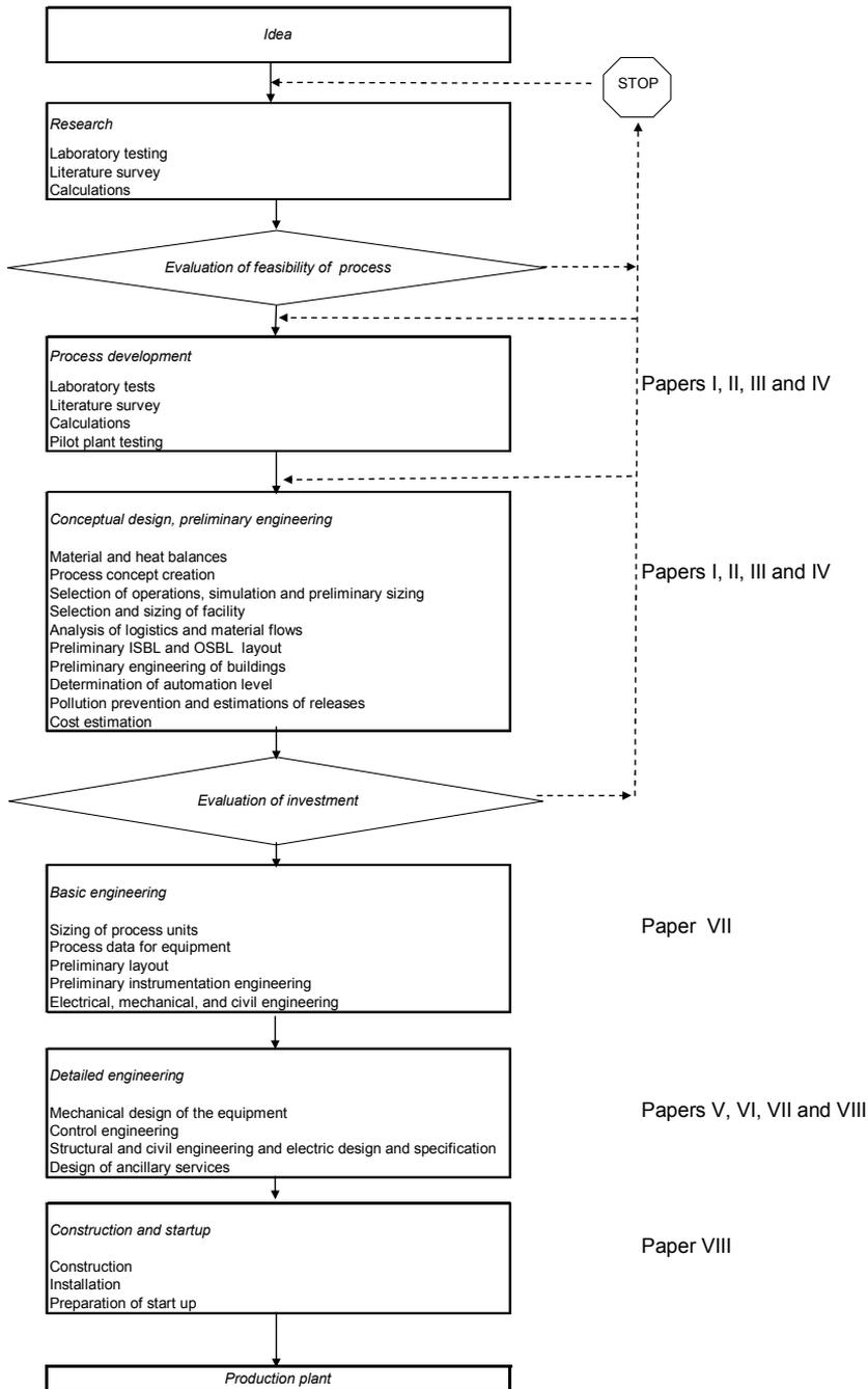
Figure 1. Process design stages (based on Aittomäki et al. 2002). Steps where the methods presented in Papers I to VIII can be applied are also pointed out.
